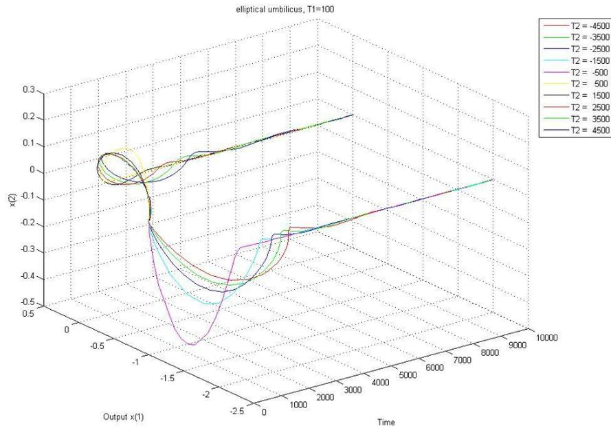
**Figure 2.** Behavior of output of designed control system in the case of integrators in series at various  $T_2$ .
