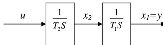
**Figure 1.** “Integrators in series” structure.
