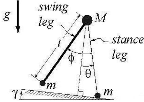
**Figure 9.** Double pendulum with slope
