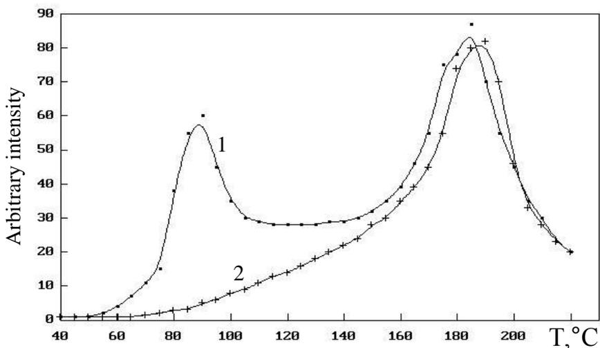
Figure 1. TL curves of irradiated crystal LiF-U at 300 K:
