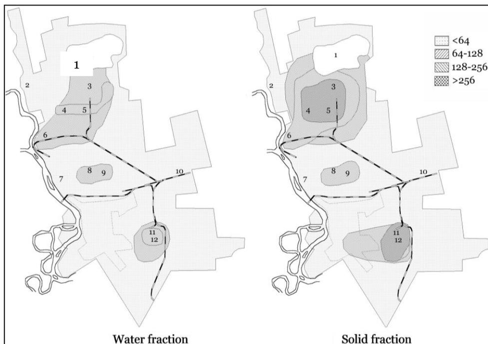
**Figure 1.** Map-scheme of the total contamination coefficient ( $Z_c$ ) in water, solid fractions of snow cover in Pavlodar (mg/kg). 1 – sump of Balkyldak lake; 2 – Pavlodarskoe village; 3 – Pavlodar chemical plant; 4 – Pavlodar petrochemical plant; 5 – CHP-3; 6 – Zhana-aul village; 7 – Lesozavod village; 8 – Pavlodar tractor plant; 9 – CHP-2; 10 – Zhetekshi village; 11 – Pavlodar aluminum plant; 12 – CHP-1
