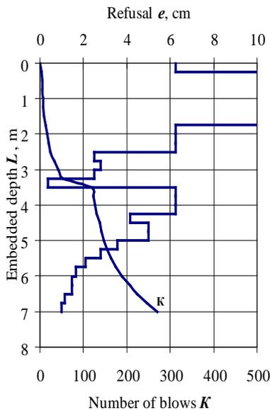
Fig. 3 Graphics before pile length increasing for testing pile LT1
