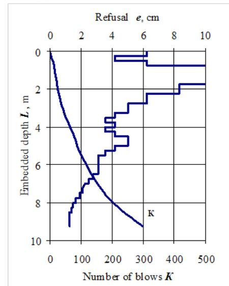
Fig.6 Graphics before pile length increasing for testing pile LT4
