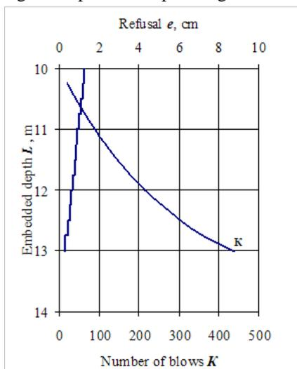
Fig. 9 Graphics after pile length increasing, LT3
