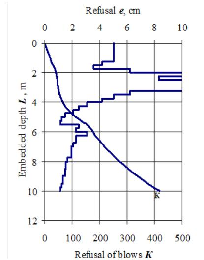
Fig. 5 Graphics before pile length increasing for testing pile LT3
