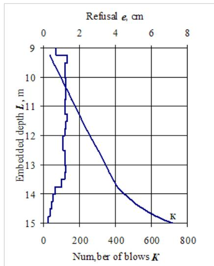
Fig. 8 Graphics after pile length increasing, LT2
