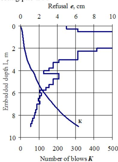
Fig. 4 Graphics before pile length increasing for testing pile LT2
