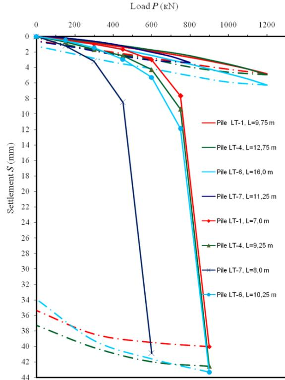
Fig.12 Correlation between settlement S and load P, the results of field static tests on piles after increasing
