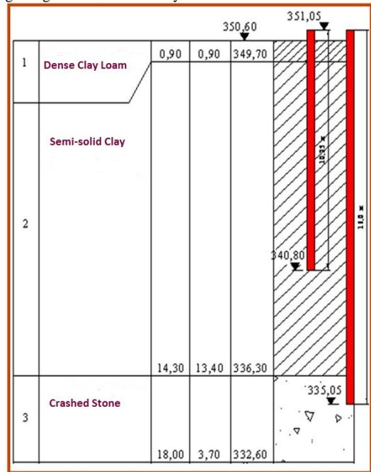
Fig. 2 Geology of the construction site of the USA Embassy in Astana
