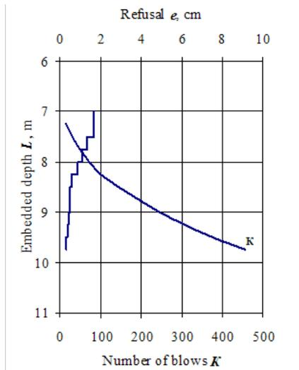
Fig. 7 Graphics after pile length increasing, LT1
