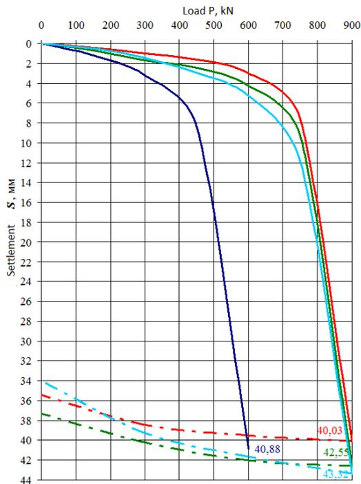
Fig.11 Correlation between settlement S and load P, the results of field static tests on piles before increasing
