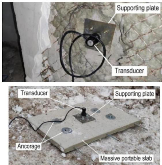
**Fig. 2.** Vibration monitoring sensors.
