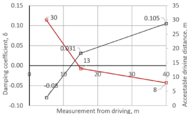
**Fig. 8.** Allowable distancing of the pile driving site.
