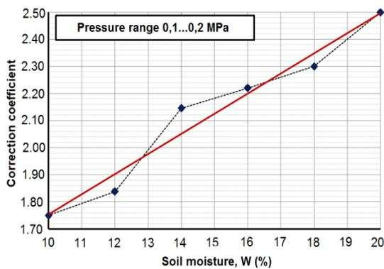
Fig.12 Correction factors for reduction for loamy soils (0.1-0.2 MPa)
