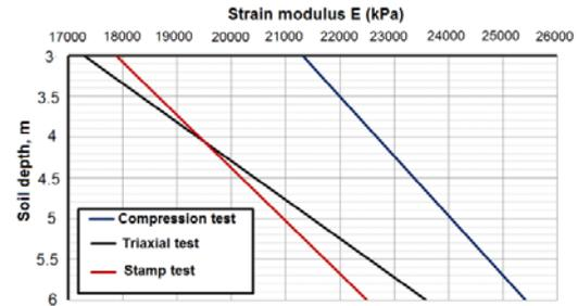
Fig.11 Comparison of deformation modulus for sandy soil obtained by various tests
