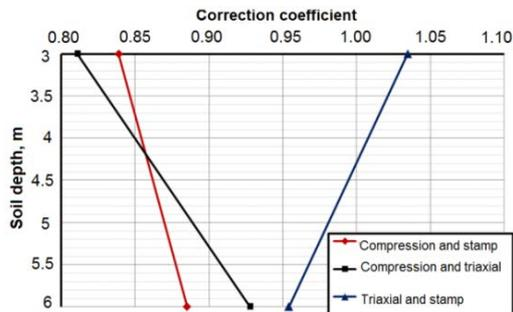
Fig.16 Correction factors for reduction of the compression modulus for sandy soils
