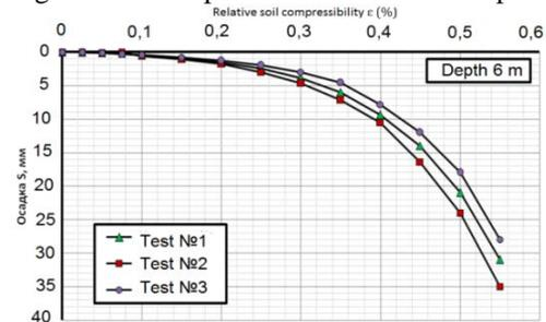
Fig.8 Results of plate-load tests at 6 m depth (sandy soils)
