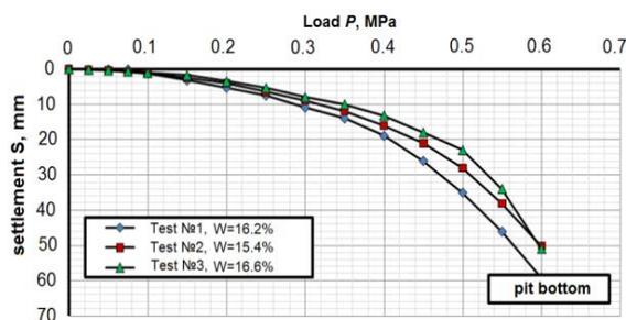
Fig.6 Results of plate-load tests at 1 m depth (loamy soils)
