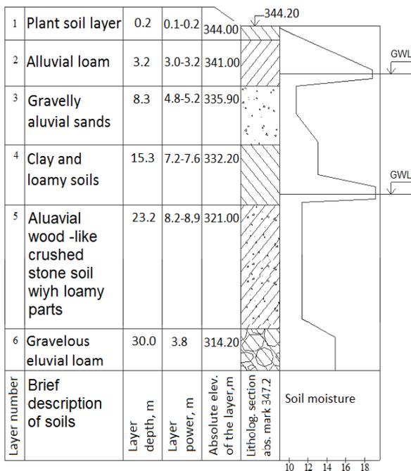
Fig.1 Profile of the construction site
