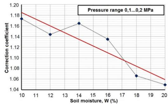
Fig.14 Correction factors for reduction for loamy soils (0.1-0.2 MPa)
