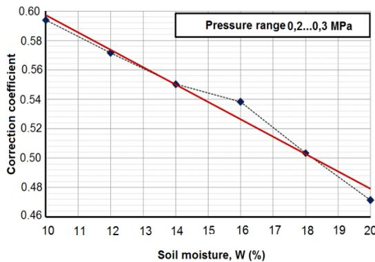
Fig.13 Correction factors for reduction for loamy soils (0.2-0.3 MPa)
