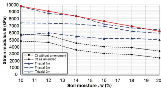
Fig.9 Comparison of deformation modulus for loamy soil obtained by various tests (0.1-0.2 MPa)
