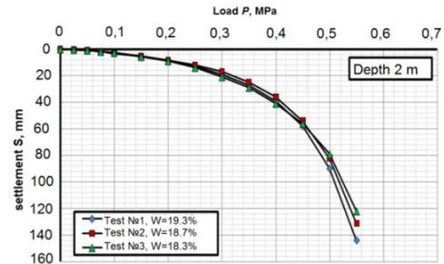
Fig.7 Results of plate-load tests at 2 m depth
