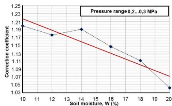
Fig.15 Correction factors for reduction of the stabilometric modulus of deformation to the plate-load ones for loamy soils (0.2-0.3 MPa)
