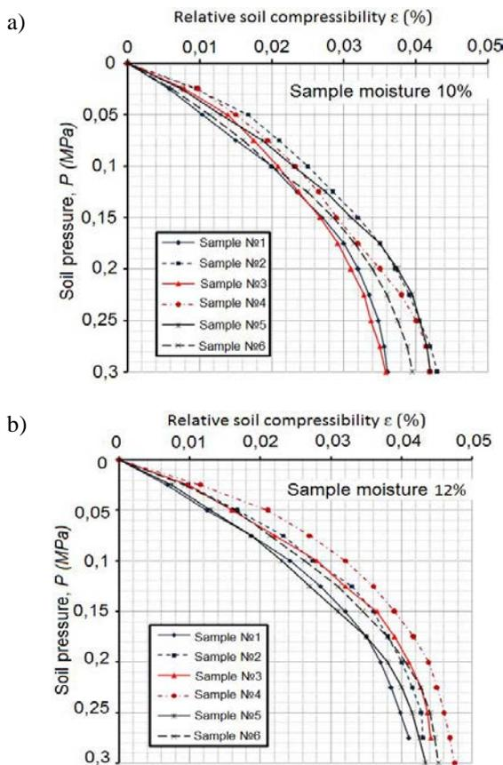
Fig.2 Results of compression tests of loamy soil samples with water content: a) 10%; b) 12%
