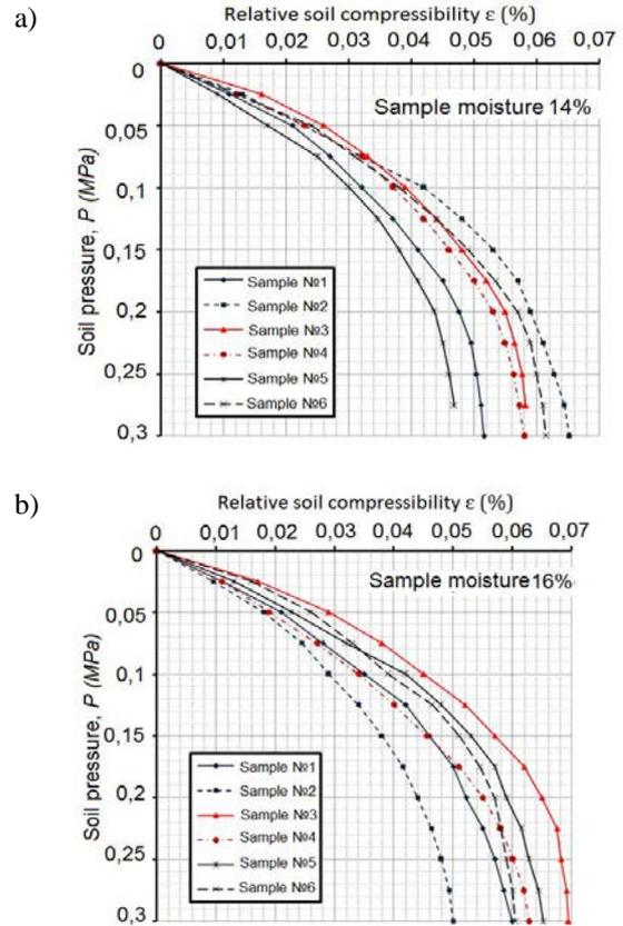
Fig.3 Results of compression tests of sandy soil samples with water content: a) 14%; b) 16%
