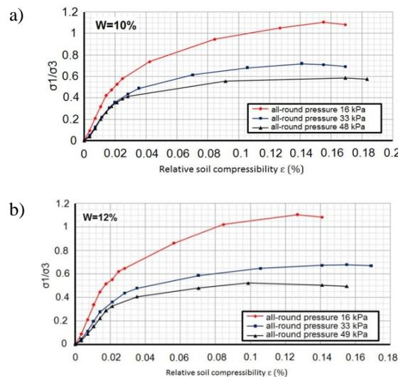
Fig. 4 Results of stabilometer tests of loamy soil samples with water content: a) 10%; b) 12%
