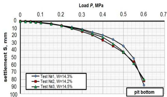
Fig.5 Results of plate-load tests of soils from the excavation pit bottom (loamy soils)
