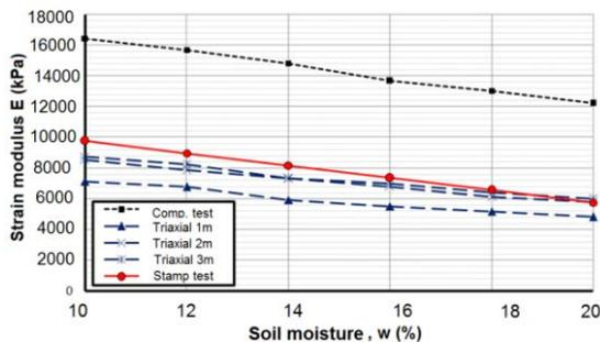
Fig.10 Comparison of deformation modulus for loamy soil obtained by various tests (0.2-0.3 MPa)
