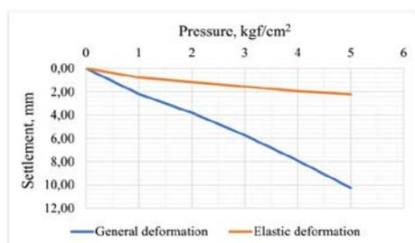
Fig. 6 Results of Point 1.1 (wet soil)
