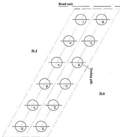
Fig.11 Pile plan field
