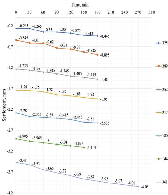
Fig. 16 Graph of results of the settlement of the pile No. 16 by loading stages
