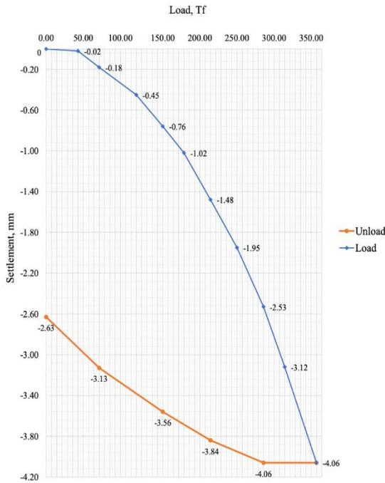
Fig. 15 Graph of results of the total settlement of the pile No. 16
