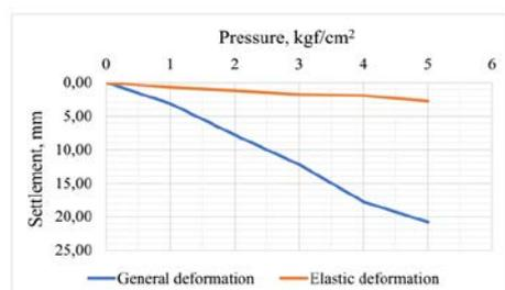
Fig. 8 Results of Point 2.1 (wet soil)
