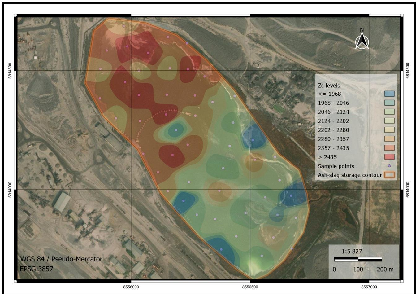
**Fig 3. 2D spatial distribution of Zc levels on the ash-slag storage of AFP.** Coordinate system: WGS 84: Pseudo-Mercator EPSG: 3857, satellite map: ESRI Satellite [ArcGIS/World\_Imagery], scale: 1:5827, method of interpolation: QGIS IDW, distance coefficient = 5.0, pixel size = 0.275182.
