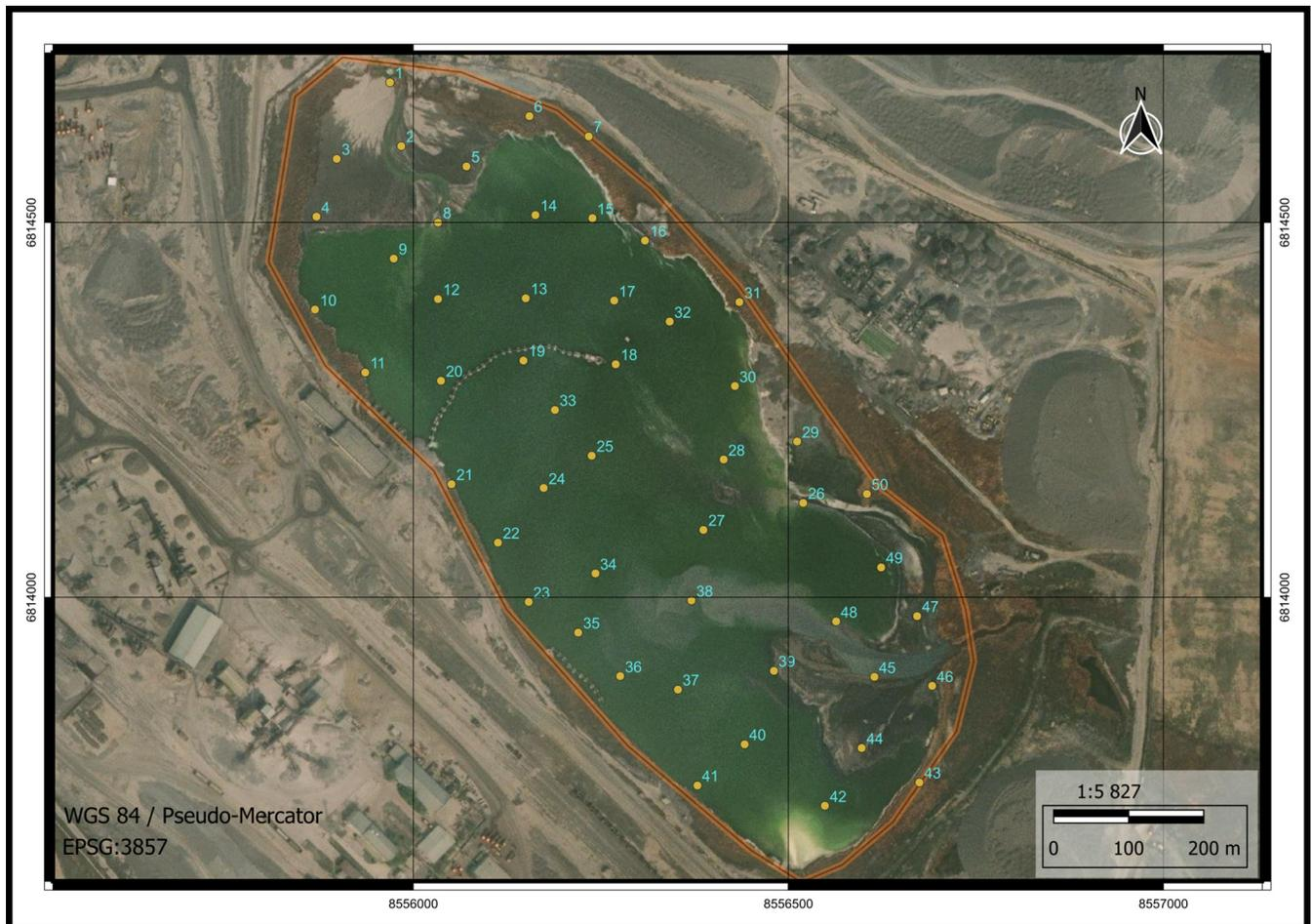
**Fig 1. Sampling map of ash slug storage at the Aksu Ferroalloy Plant [Aksu, Kazakhstan].** Coordinate system: WGS 84: Pseudo-Mercator EPSG: 3857, satellite map: ESRI Satellite [ArcGIS/World\_Imagery], scale: 1:5827.
