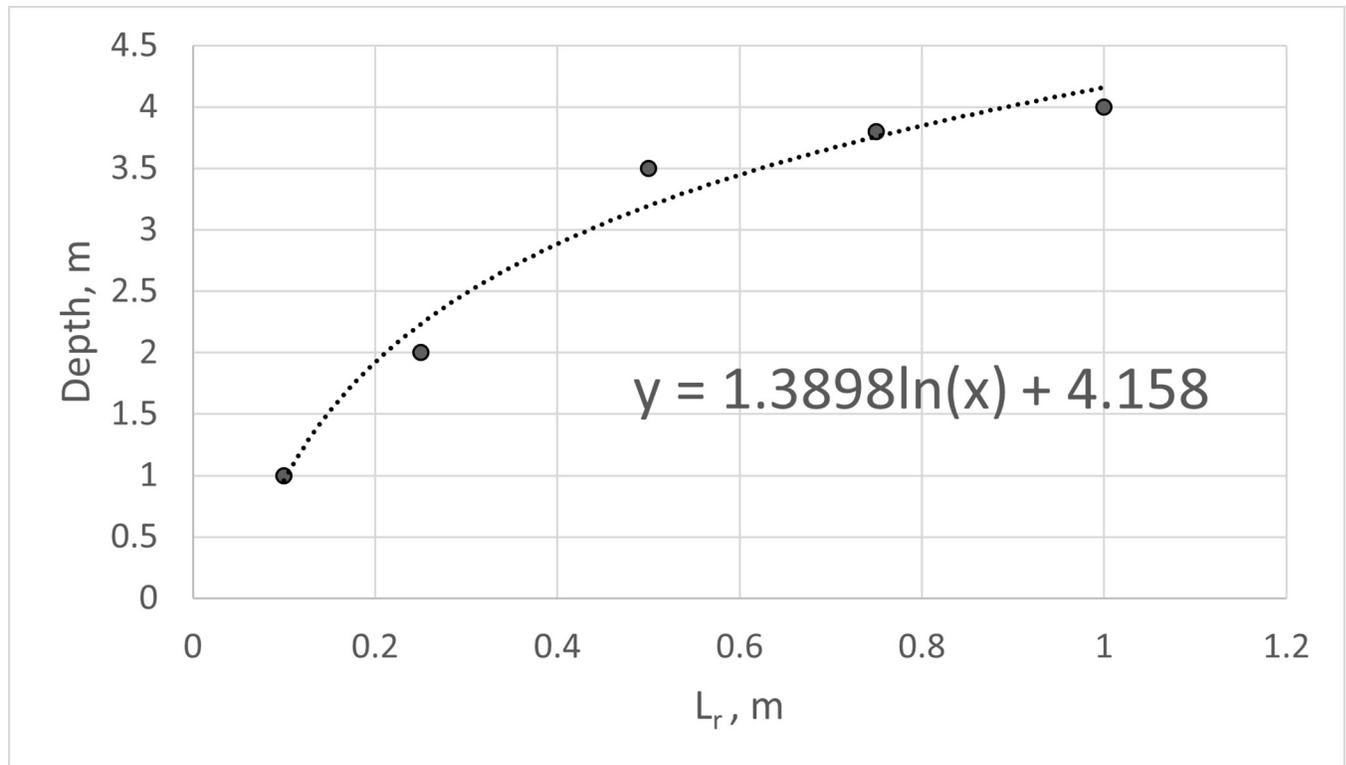
**Fig 9.** The curve of the dependence of the depth on the relative distance from the nearest zero point [Lr].
