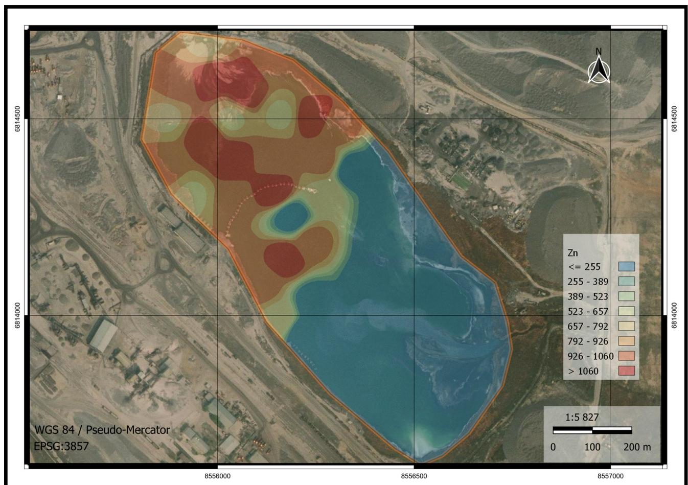
**Fig 5. Spatial distribution of Zn on the ash-slag storage of AFP.** Coordinate system: WGS 84: Pseudo-Mercator EPSG: 3857, satellite map: ESRI Satellite [ArcGIS/World\_Imagery], scale: 1:5827, method of interpolation: QGIS IDW, distance coefficient = 5.0, pixel size = 0.275182.
