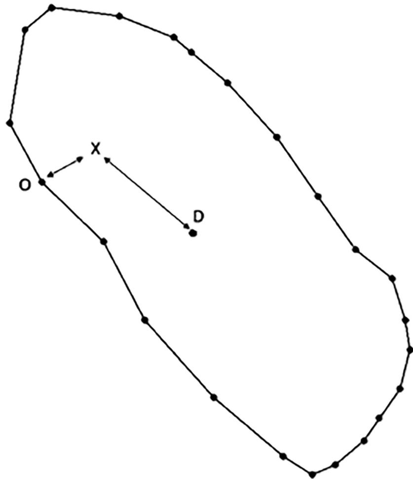
**Fig 8. Contour of an excavation with marked zero points [on the edge] and the point of the greatest depth [point D].**
