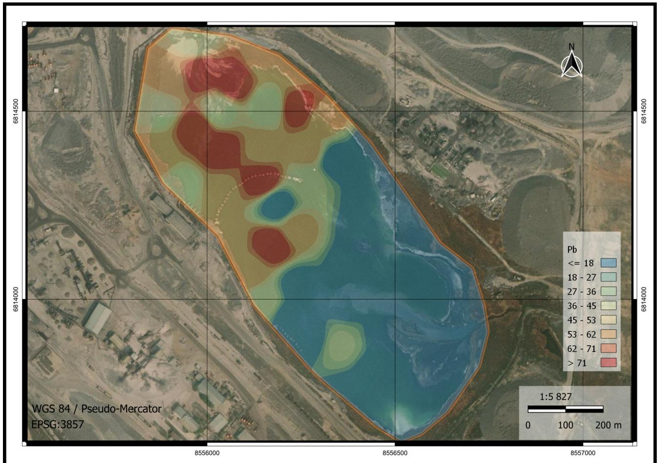
**Fig 4. Spatial distribution of Pb on the ash-slag storage of AFP.** Coordinate system: WGS 84: Pseudo-Mercator EPSG: 3857, satellite map: ESRI Satellite [ArcGIS/World\_Imagery], scale: 1:5827, method of interpolation: QGIS IDW, distance coefficient = 5.0, pixel size = 0.275182.
