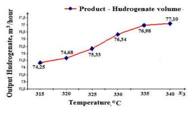
$x_1 = 80 \text{ m}^3/\text{h} - \text{input of raw material}; x_2 = 30 \text{ kg/cm}^2 - \text{pressure in R-1 reactor}; x_4 = 3 \text{ h}^{-1} - \text{volumetric raw feed rate}; x_5 = 400 \text{ nm}^3 - \text{hydrogen containing gas circulation.}$
