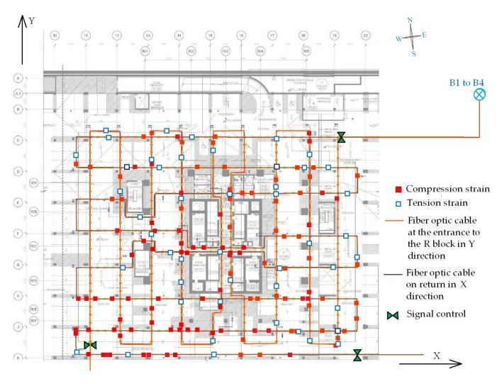
**Figure 11.** Fiber optic strain along the cable layout in block R, level B4.
