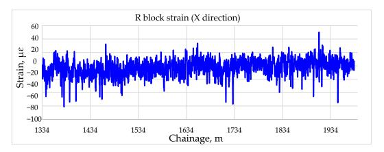
Figure 10. Strain in the X direction in the B4 raft of block R.
