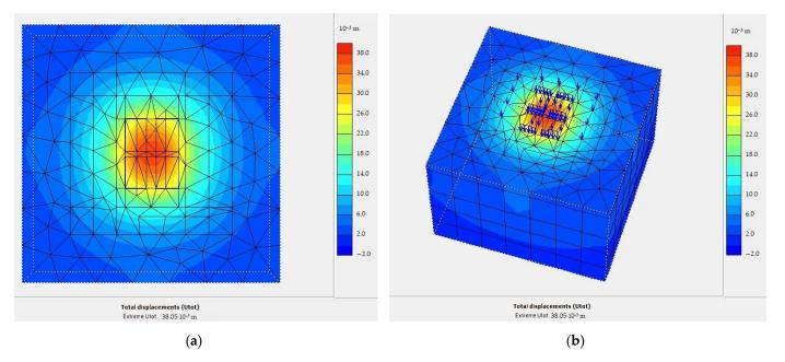
Figure 15. Settlement in vertical Z-direction: (a) view of the surface of the raft; (b) volumetric model.
