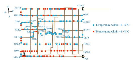
Figure 8. Temperature field distribution in block R.
