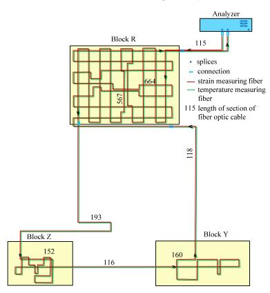
Figure 6. Schematic diagram of distributed fiber optic strain sensing system.
