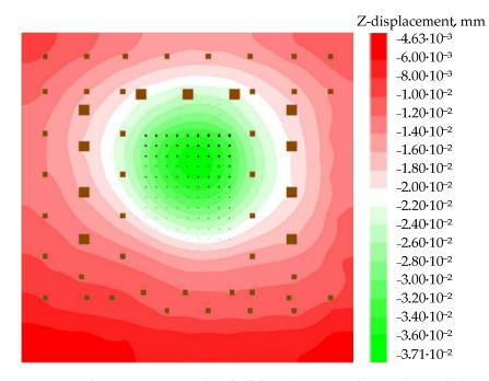
**Figure 2.** Deformation contour plan of raft foundation according to Zhussupbekov et al. [2] simulation results with FLAC 3D program.
