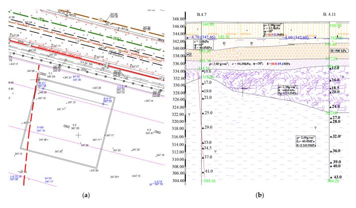
Figure 4. Construction site: (a) survey plan; (b) engineering-geological profile.
