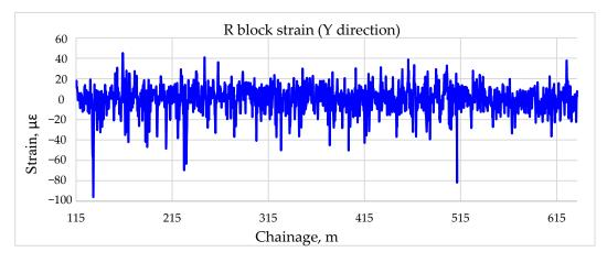
Figure 9. Strain in the Y direction in the B4 raft of the 75-storey block R building.
