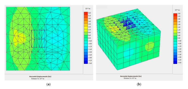
**Figure 16.** Horizontal displacement in the X-direction: (**a**) view of the surface of the raft; (**b**) volumetric model.
