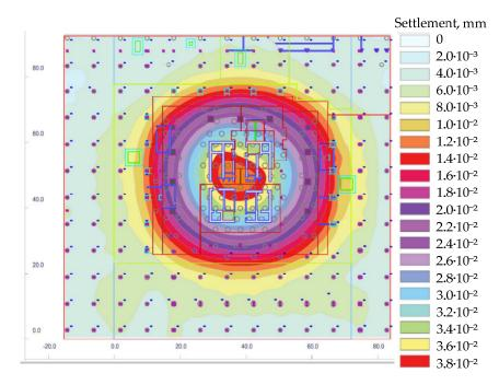
**Figure 1.** Vertical deformation plan of raft foundation according to the simulation of Buranbayeva et al. [1] using GARP software.
