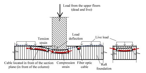
Figure 17. Strains near point loads (columns).
