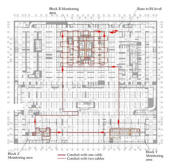
Figure 5. Part plan of cable routing in Block R monitoring area on B4 raft.
