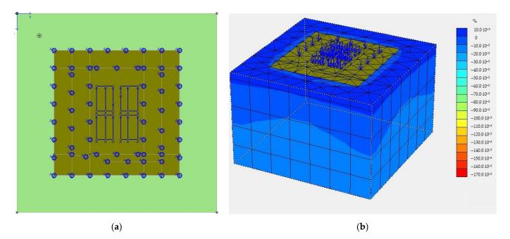
Figure 14. Numerical modeling in Plaxis 3D: (a) loading scheme; (b) volumetric strains.
