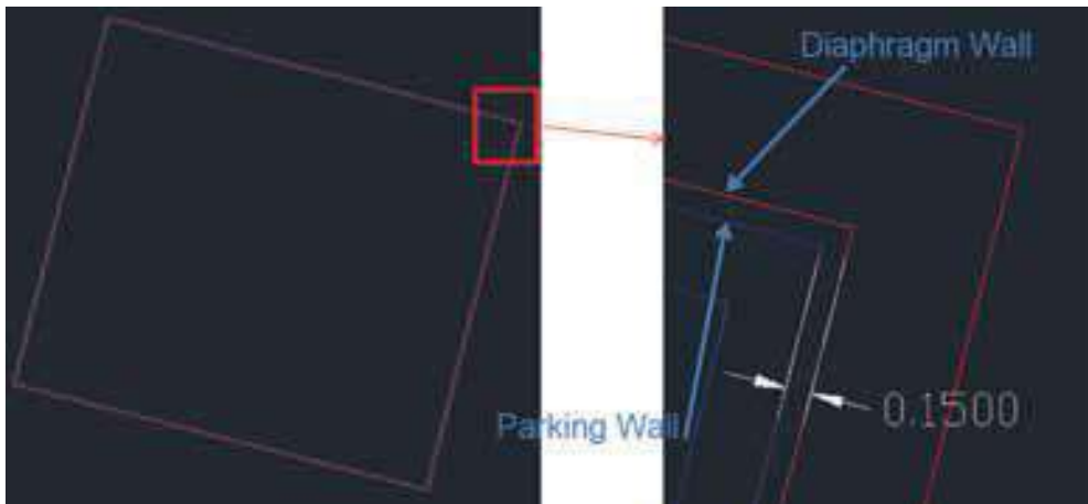
Figure 2: Diaphragm wall position in comparison with the inner wall
