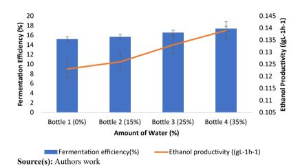
Figure 4. Effect of water content variation on fermentation efficiency and ethanol production of cassava peels in the laboratory studies
