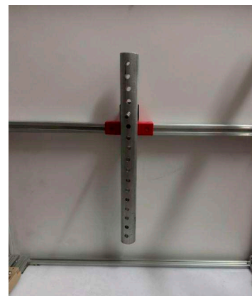
Fig. 3. General view of a laboratory setup for studying the law of motion of a physical pendulum
