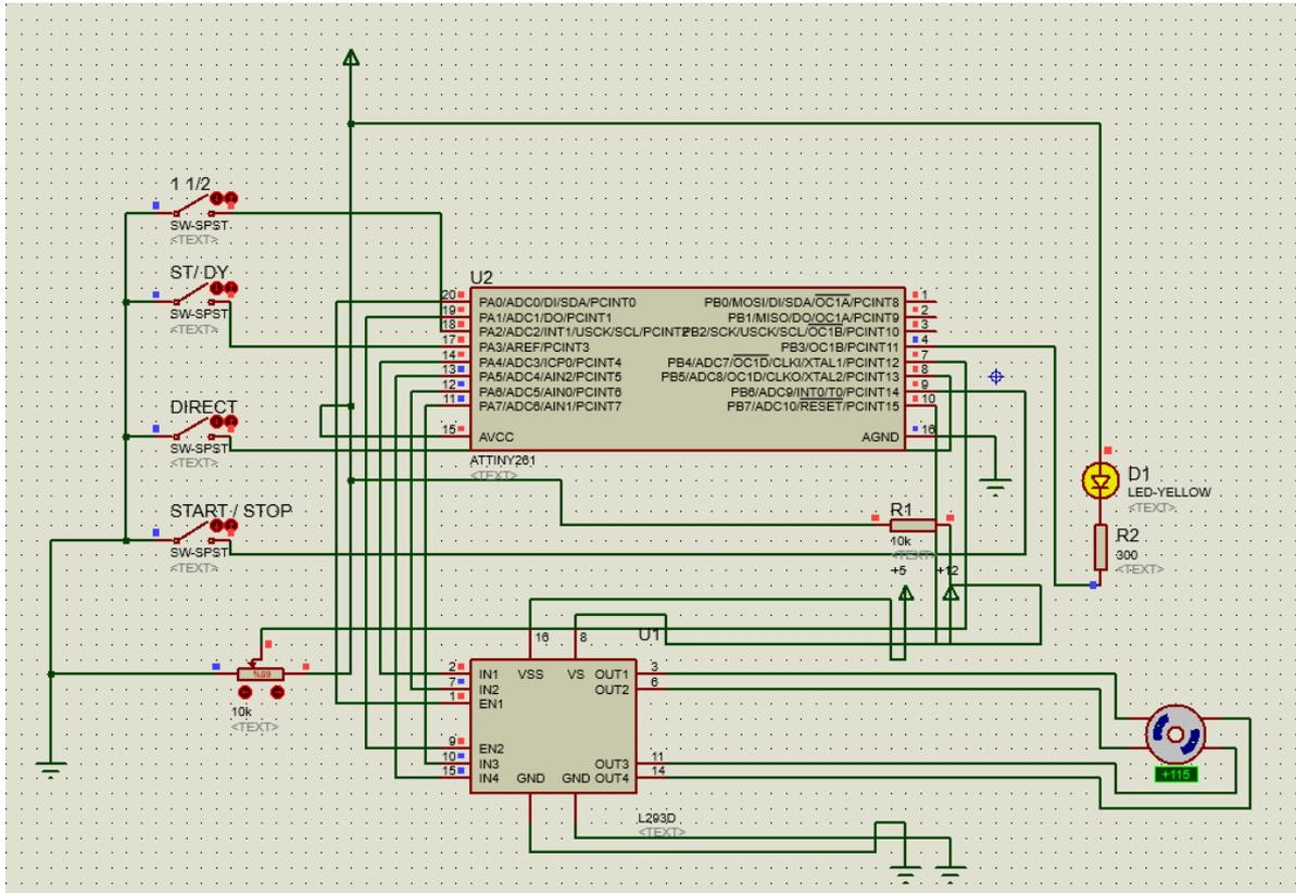
Figure 2. Simulation of a stepper motor in the Proteus programming environment
