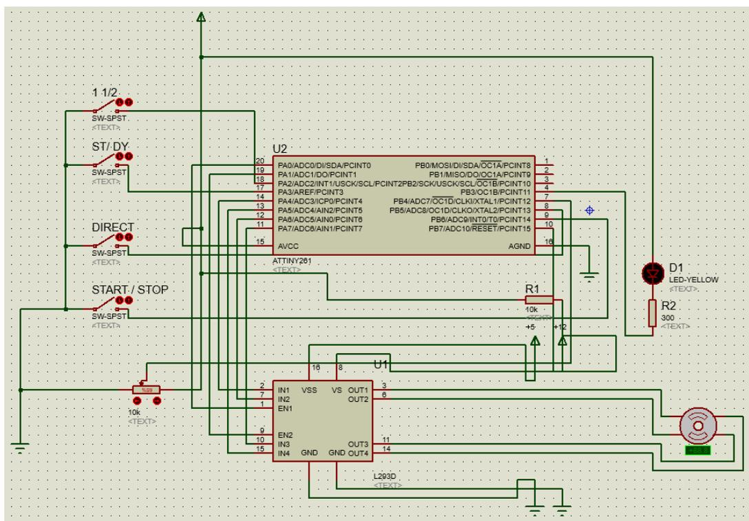
Figure 1. Schematic diagram of the bipolar stepper motor driver
