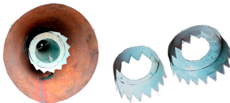
Figure 6. General view of cylindrical nozzles ( d_1 = 120 mm, d_2 = 150 mm).
