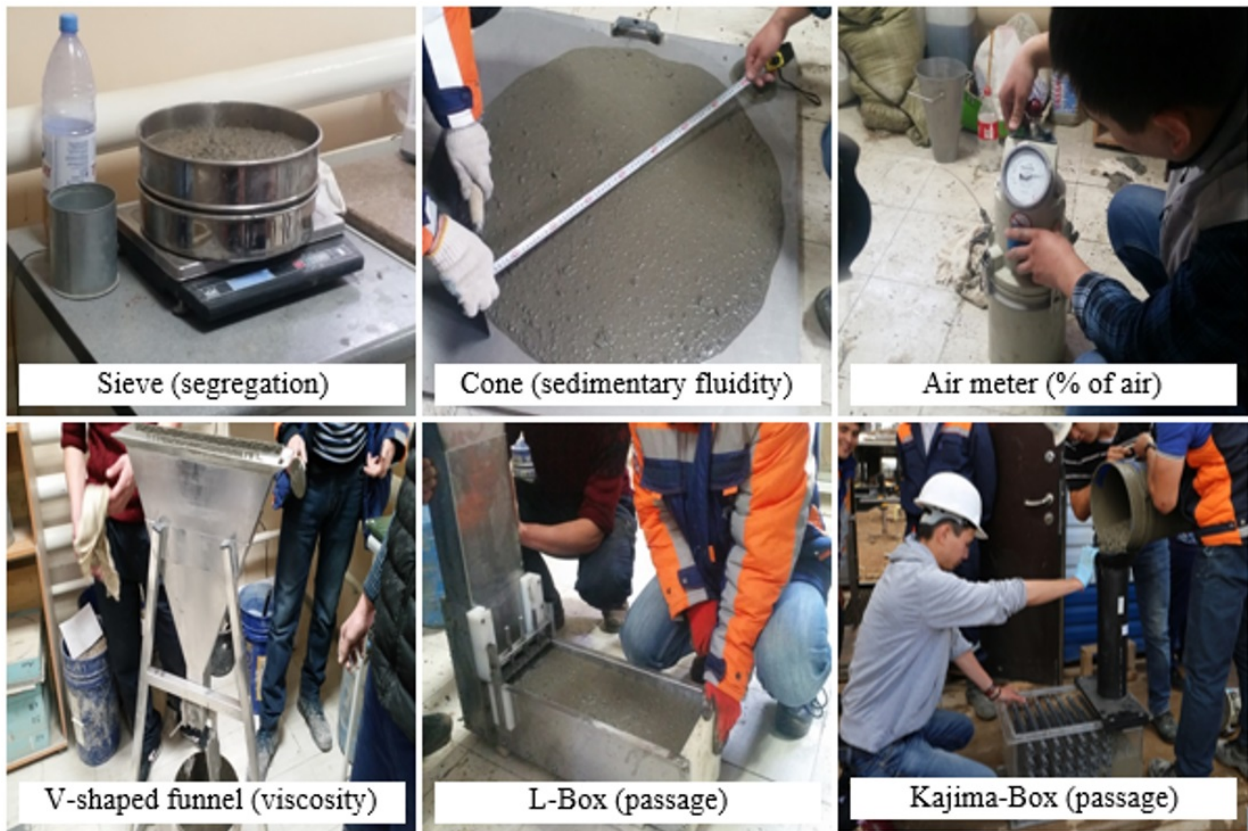
FIGURE 2 – Laboratory tests of SCC mixture
