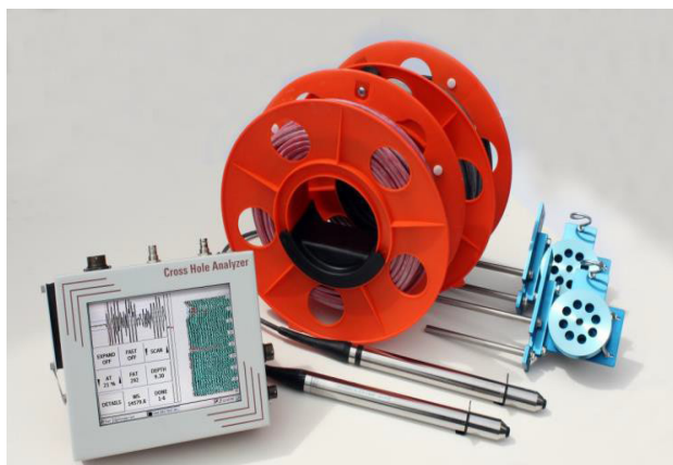
Figure 5. Cross-Hole Sonic measuring device – CHAMP: computer, cable, depth encoders, test probes
