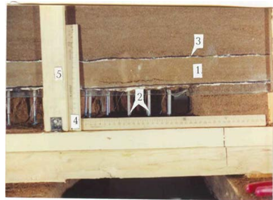
Fig.6 Model: bottom view 1–sandstone layer, 2–artificial struts, 3–layering line, 4–measuring rulers, 5–model strut
