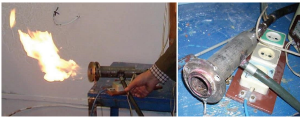
FIGURE 4: Cross jet gas burner in operation.
