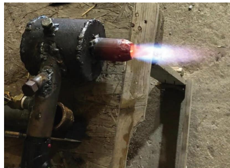
FIGURE 2: Swirl burner device in operation.
