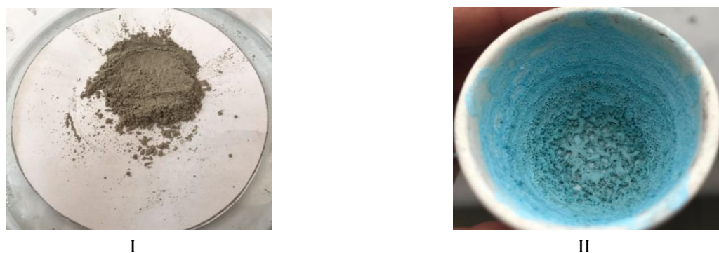
Figure 1. The slag dispersed of the metallurgical enterprise “Arcelor Mittal Temirtau” (I); sorbent obtained after alkaline treatment (II)
