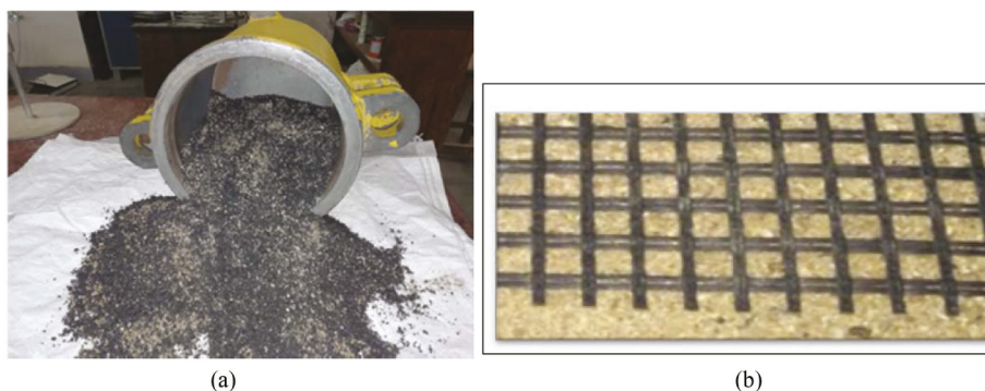
Figure 1. (a) Typical sand-rubber mixture sample (b) Geogrid used for the study.
