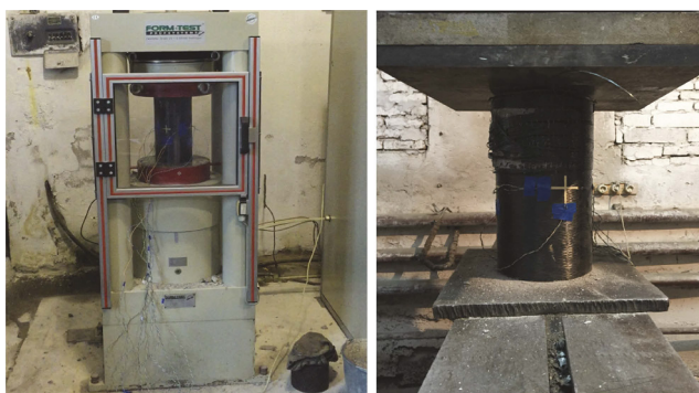
Figure 1. General view of the test of reinforced samples for axial compression on hydraulic presses ALPHA 3-3000S and IPS-200.
