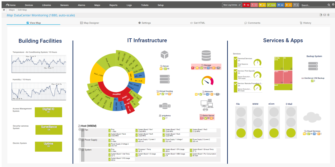
Figure 1. Example of the PRTG network monitoring system information panel.
