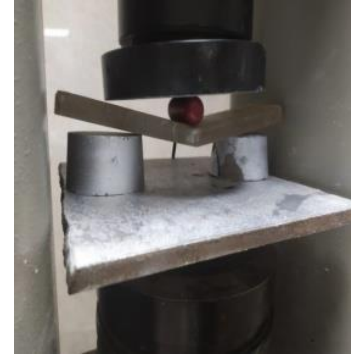
Figure 7. Testing the composite specimen on the hydraulic press
