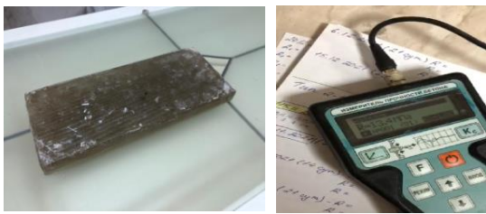
Figure 6. Photos of the obtained polymeric material and the device for measuring the strength of materials
