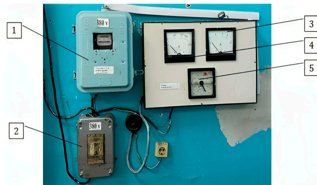
Figure 1. Measuring stand for determining the energy characteristics of a screw press. 1—electricity meter; 2—switch; 3—ammeter; 4—voltmeter; 5—phase meter.
