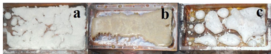
Figure 7. Photographs of activated W samples of \text{BaF}_2 (a), \text{MgF}_2 (b), and \text{BaMgF}_4 (c) ceramics synthesized under the influence of an electron beam with E = 1.4 MeV, P = 15 \text{kW}/\text{cm}^2 , R1.
