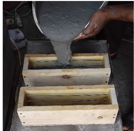
Fig. 1a. Placing of specimens.
