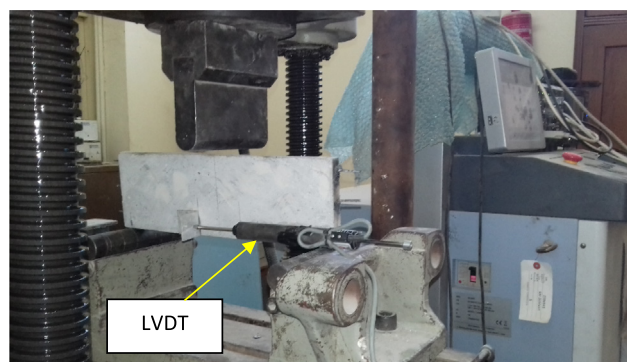
Fig. 1d. Crack creation under three-point loading.
