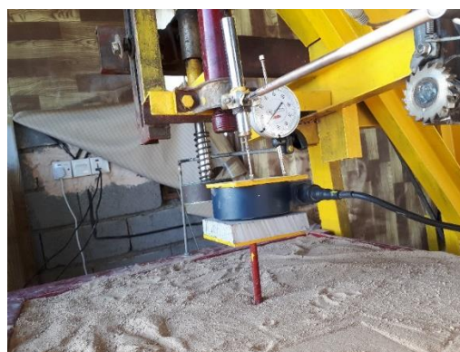
Figure 8. Loading system of screw pile and gauges.
