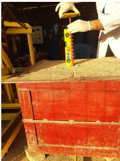
Figure 6. Insertion of screw pile in soil.
