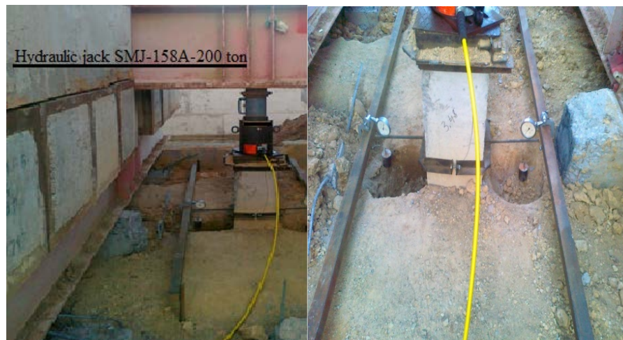
Figure 6. SLT of the piles
