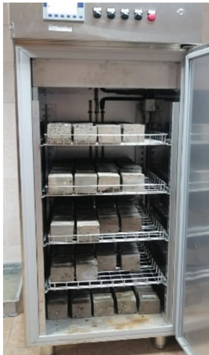
Figure 4. View of typical cubes in climate chamber before first FnT cycle.
