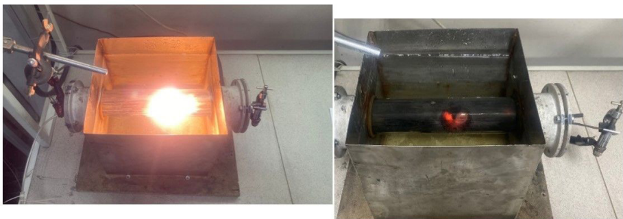
Figure 4. Installation for the extraction of carbon nanomaterial using the electric arc method.
