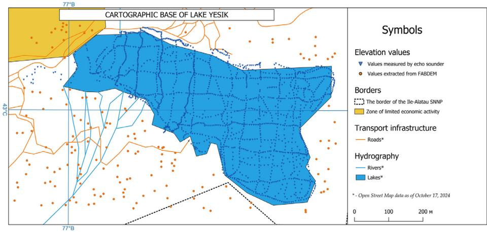
**Fig. 2.** Combined data for the analysis of the bottom relief of Lake Yesik.
