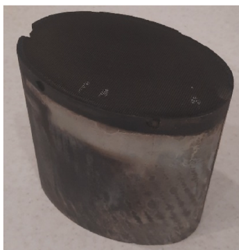
Fig. 5. A used 1995 Toyota Mark II catalytic converter with 200,000 km mileage (gasoline).
