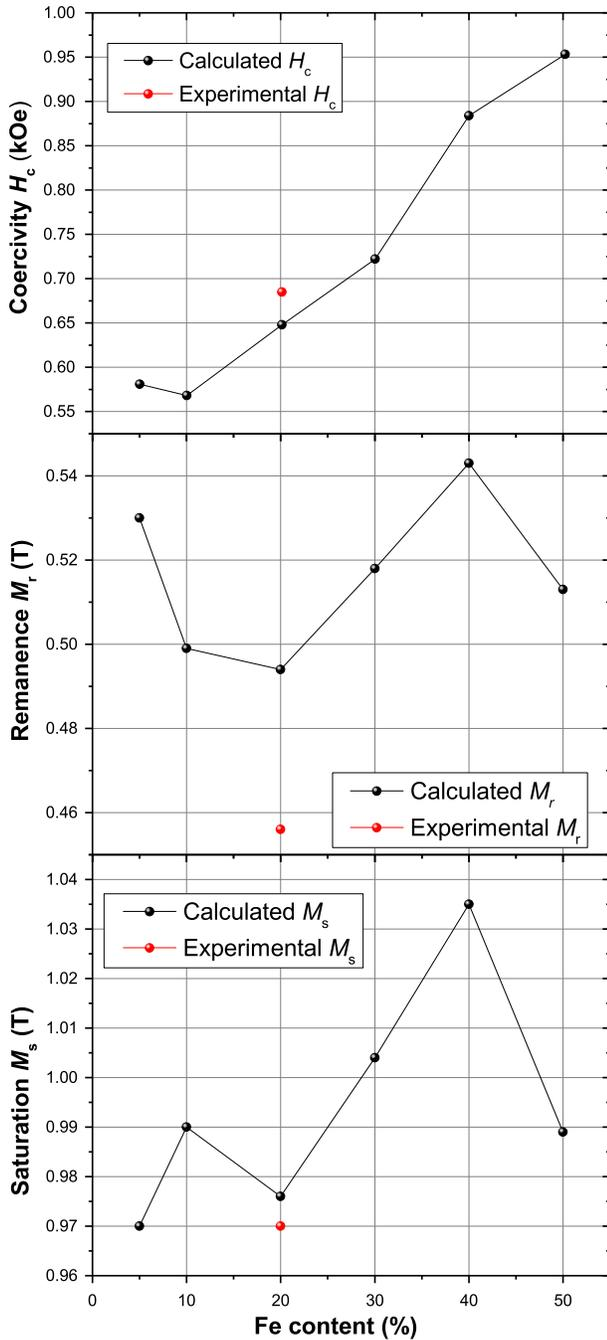
Fig. 6. Dependence of magnetic characteristics on iron content in the Fe/Fe<sub>3</sub>O<sub>4</sub> system from calculated and experimental data.
