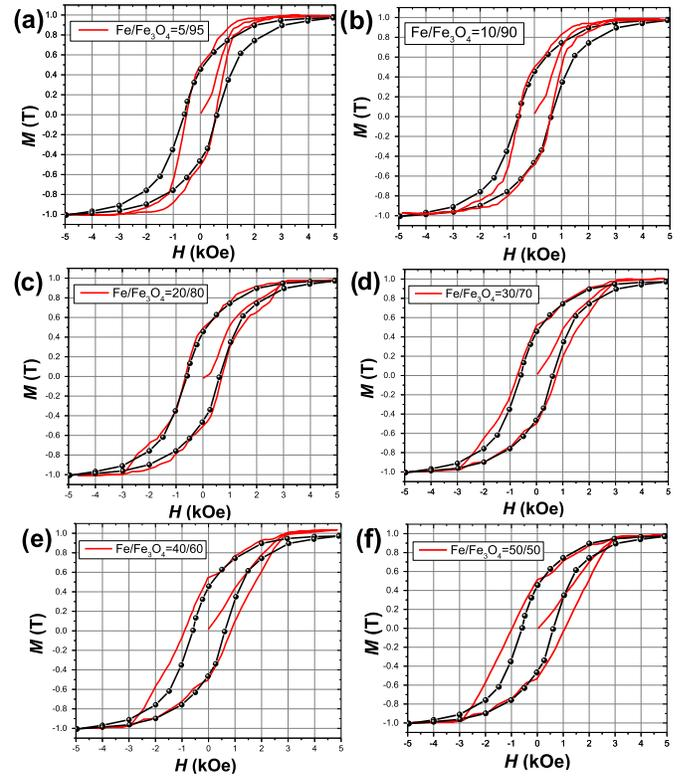
Fig. 5. Comparison of hysteresis loops for different Fe/Fe<sub>3</sub>O<sub>4</sub> contains. The black points are experimental data obtained for 20%Fe + 80%Fe<sub>3</sub>O<sub>4</sub> press compact and the red lines are calculated loops using a PMRM program, based on the change in the phase ratio (in %) for Fe/Fe<sub>3</sub>O<sub>4</sub>: (a) 5/95, (b) 10/90, (c) 20/80, (d) 30/70, (e) 40/60, and (f) 50/50.
