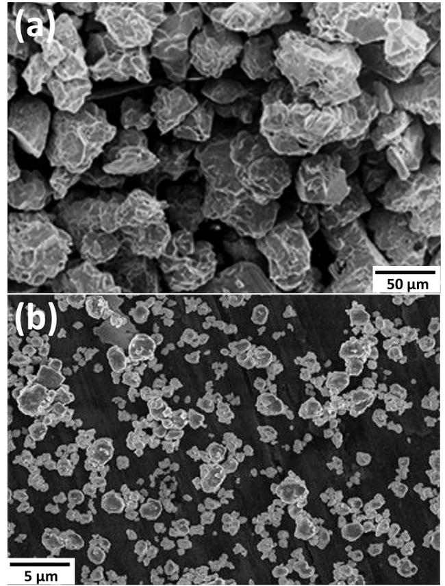
Fig. 3. SEM images (a) initial sample and (b) sample processed in high-energy mill during 4 h.
