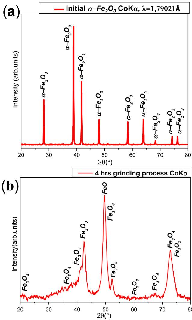
Fig. 4. XRD patterns (a) initial sample and (b) sample processed in high-energy mill during 4 h.
