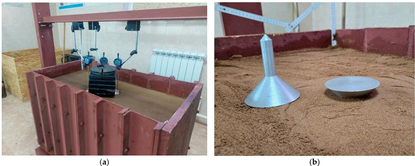
**Figure 6.** Laboratory testing in the expandable box: (a) static loading; (b) testing models.
