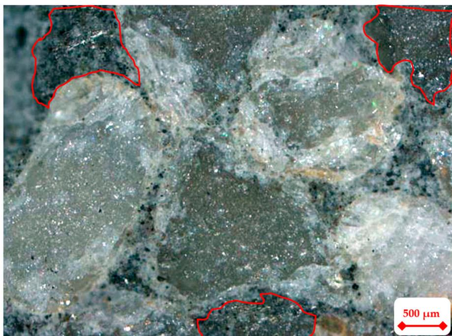
**Figure 6.** Microstructure of SCC with microsilica (magnification of 500  $\mu\text{m}$ ).
