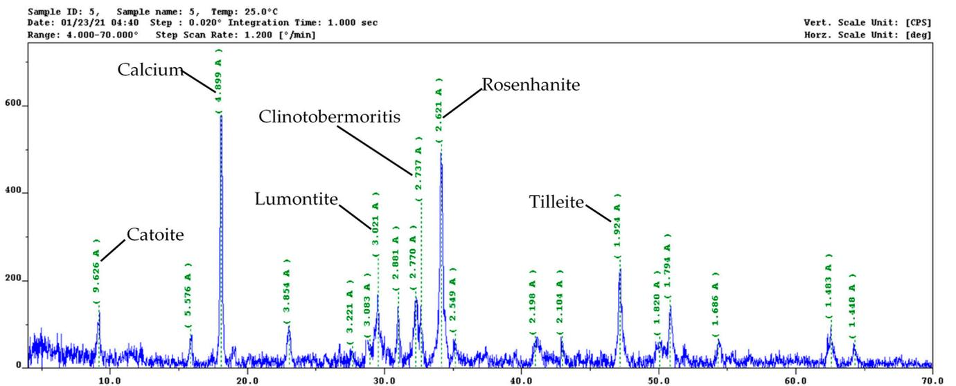
Figure 9. Sample with replacement of part of cement with opoka.
