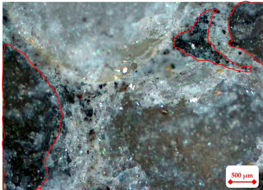
**Figure 5.** Microstructure of SCC on metakaolin (magnification of 500 μm).
