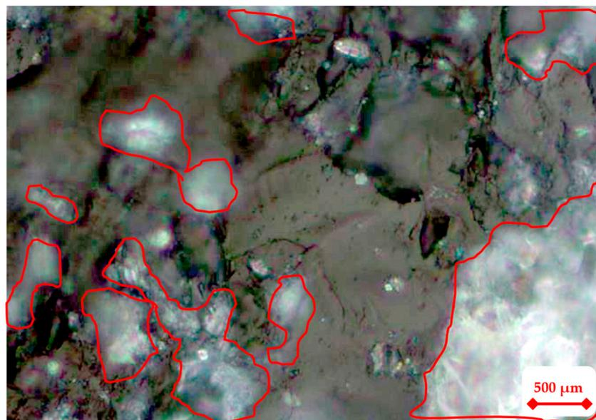
**Figure 3.** Microstructure of SCC made from pure cement (magnification of 500  $\mu\text{m}$ ).
