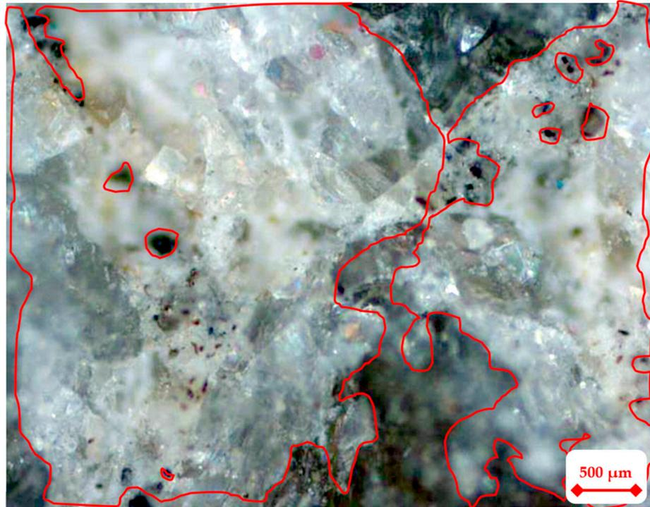
**Figure 4.** Microstructure of SCC with opoka (magnification of 500 μm).
