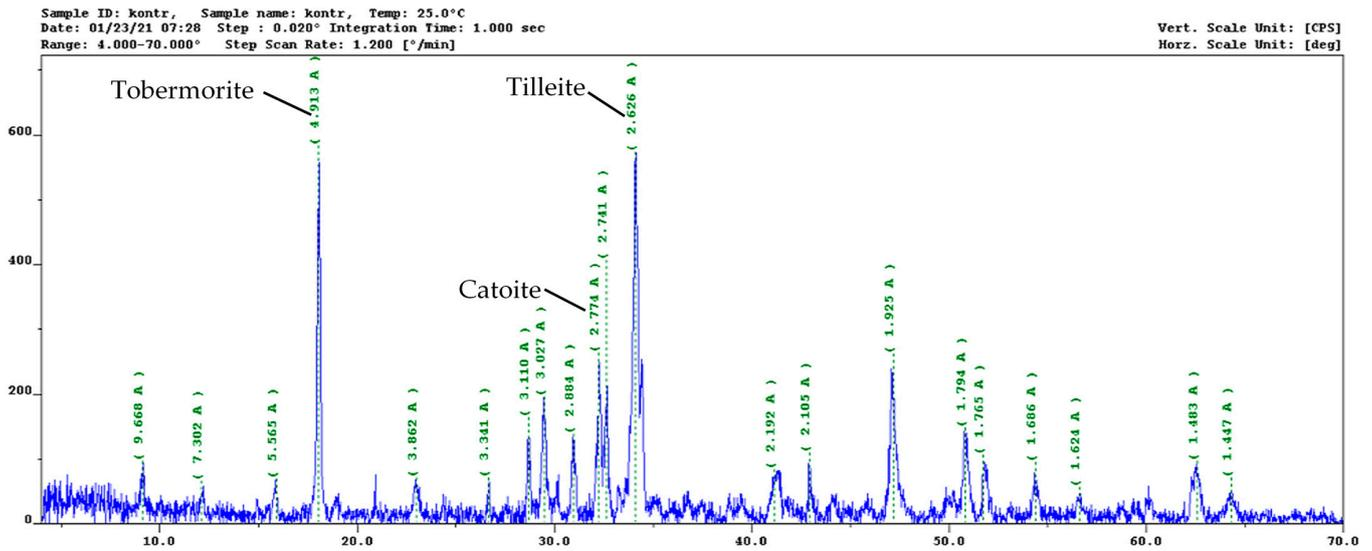
Figure 7. Reference sample without mineral additive.
