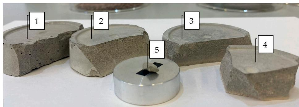
**Figure 2.** Macrostructure of SCC mortar samples: (1) without filler; (2) 5% opoka; (3) 10% metakaoline; (4) 15% microsilica; (5) sample for SEM.
