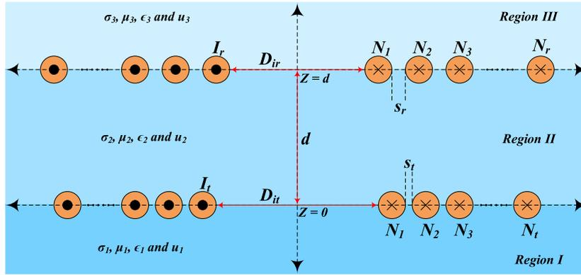
**FIGURE 1.** Region divisions and the location of coaxial circular planar coils at the boundaries in the cylindrical coordinate system.
