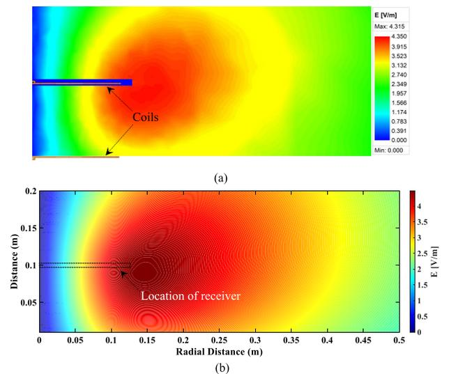
**FIGURE 14.** Electric field intensity distribution within the semi-finite water region, at the frequency of 400 kHz and applied current amplitudes of  $I_t = I_r = 5A$  (a) FEM analysis (b) Analytical modeling.
