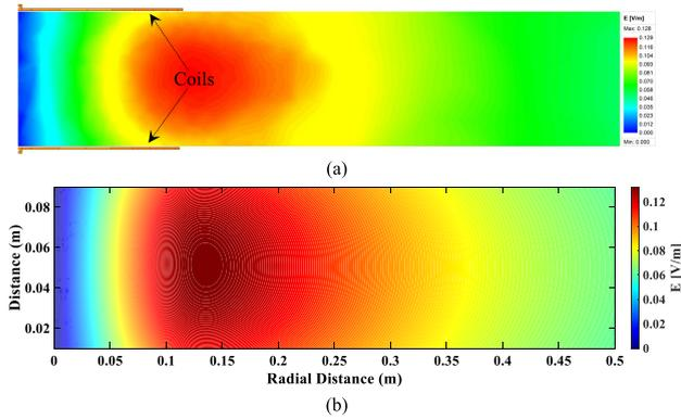
**FIGURE 15.** Electric field intensity distribution within the finite water region, at the frequency of 85 kHz and applied current amplitudes of  $I_t = I_r = 5A$  (a) FEM analysis (b) Analytical modeling.
