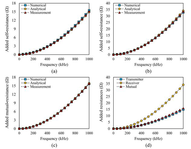
**FIGURE 4.** Additional resistances for the semi-finite medium. (a) Additional self-resistance of transmitter (b) Additional self-resistance of receiver (c) Mutual resistance (d) Overall comparison.
