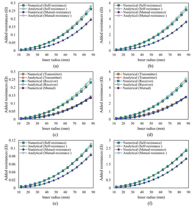
**FIGURE 8.** Comparison of the additional resistances for various values of the inner radius at the frequency of 85 kHz and 400 kHz in each specific case. (a) Infinite medium at 85 kHz (b) Infinite medium at 400 kHz (c) Semi-finite medium at 85 kHz (d) Semi-finite medium at 400 kHz (e) Finite medium at 85 kHz (f) Finite medium at 400 kHz.
