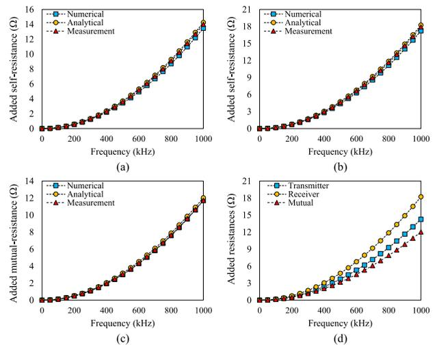
**FIGURE 5.** Additional resistances for the finite medium. (a) Additional self-resistance of transmitter (b) Additional self-resistance of receiver (c) Mutual resistance (d) Overall comparison.
