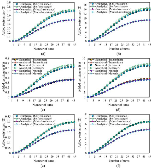
**FIGURE 6.** Comparison of the additional resistances for various number of turns at the frequency of 85 kHz and 400 kHz in each specific case. (a) Infinite medium at 85 kHz (b) Infinite medium at 400 kHz (c) Semi-finite medium at 85 kHz (d) Semi-finite medium at 400 kHz (e) Finite medium at 85 kHz (f) Finite medium at 400 kHz.
