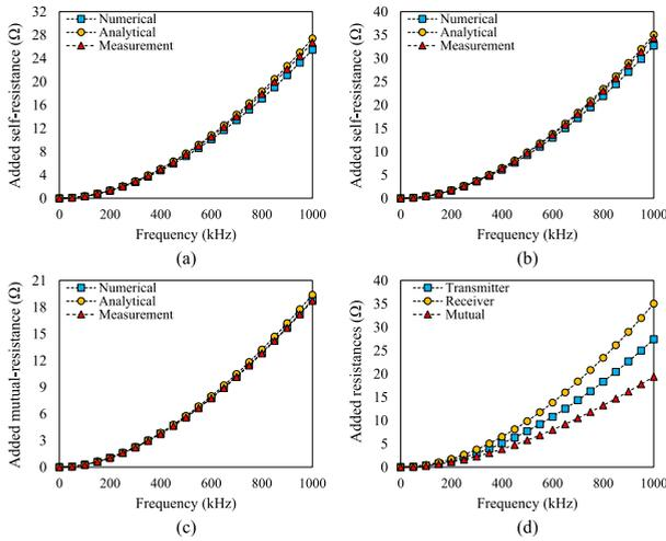
**FIGURE 3.** Additional resistances for the infinite medium. (a) Additional self-resistance of transmitter (b) Additional self-resistance of receiver (c) Mutual resistance (d) Overall comparison.
