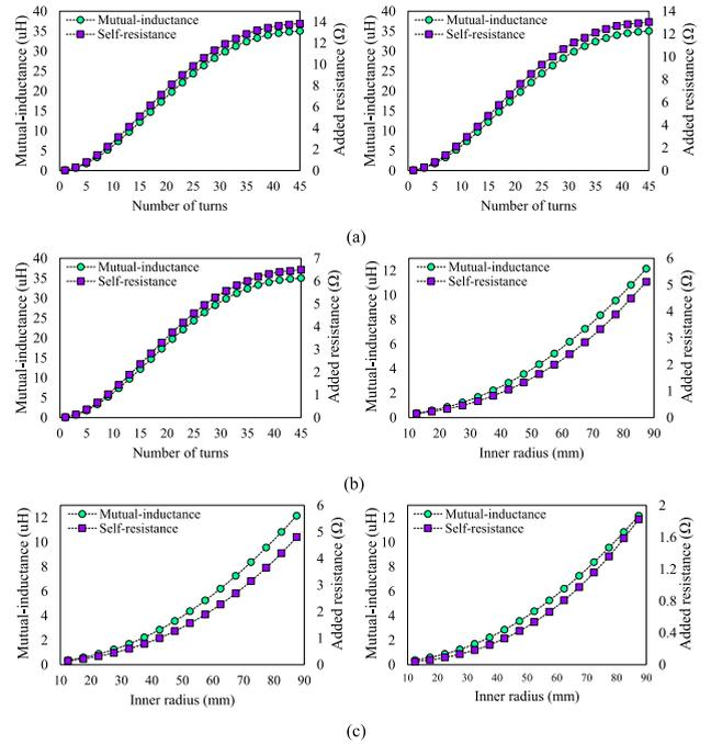
**FIGURE 10. Comparison of additional resistances and mutual inductances for different numbers of turns and inner radii at the frequency of 400 kHz for each specific case: (a) Infinite medium (b) Semi-finite medium (c) Finite medium.**
