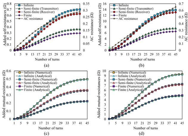
**FIGURE 7.** Additional resistances comparison for various number of turns at the frequency of 85 kHz and 400 kHz. (a) Additional self-resistances at 85 kHz (b) Additional self-resistances at 400 kHz (c) Additional mutual-resistances at 85 kHz (d) Additional mutual-resistances at 400 kHz.
