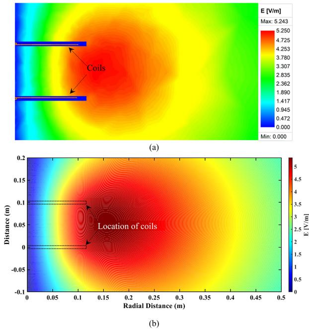
**FIGURE 12.** Electric field intensity distribution within the infinite water region, at the frequency of 400 kHz and applied current amplitudes of  $I_t = I_r = 5A$  (a) FEM analysis (b) Analytical modeling.
