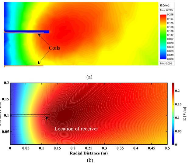
**FIGURE 13.** Electric field intensity distribution within the semi-finite water region, at the frequency of 85 kHz and applied current amplitudes of  $I_t = I_r = 5A$  (a) FEM analysis (b) Analytical modeling.
