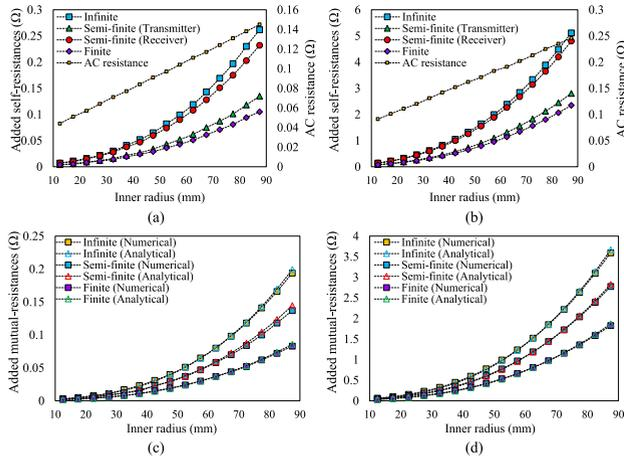
**FIGURE 9. Additional resistances comparison for various values of the inner radius at the frequency of 85 kHz and 400 kHz. (a) Additional self-resistances at 85 kHz (b) Additional self-resistances at 400 kHz (c) Additional mutual-resistances at 85 kHz (d) Additional mutual-resistances at 400 kHz.**
