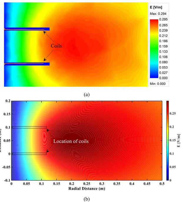
**FIGURE 11. Electric field intensity distribution within the infinite water region, at the frequency of 85 kHz and applied current amplitudes of  $I_t = I_r = 5A$  (a) FEM analysis (b) Analytical modeling.**
