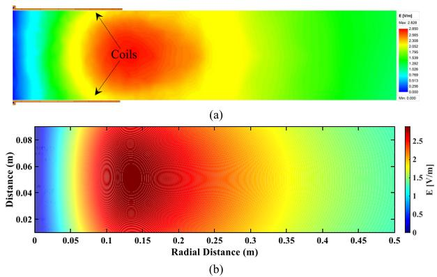
**FIGURE 16.** Electric field intensity distribution within the finite water region, at the frequency of 400 kHz and applied current amplitudes of  $I_t = I_r = 5A$  (a) FEM analysis (b) Analytical modeling.
