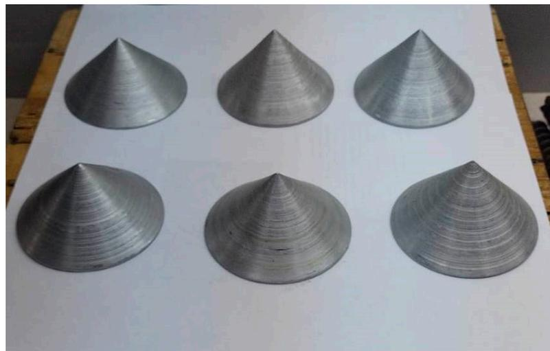
**Figure 6.** Cone foundation model.
