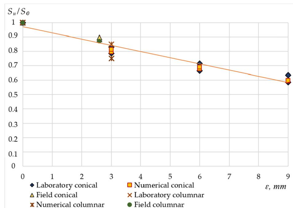
**Figure 16.** Graph of the relationship  $S_u/S_0$  depending on tensile strains based on the results of numerical, field and model laboratory tests.
