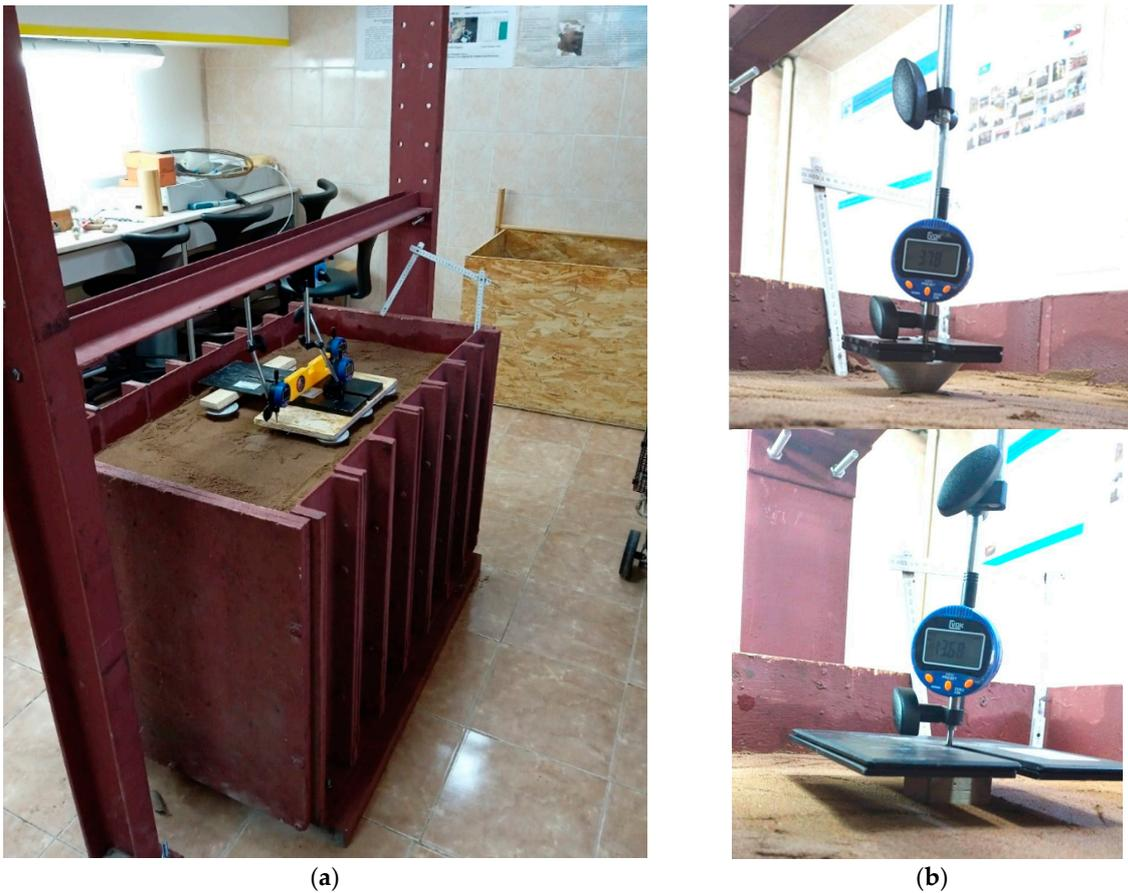
**Figure 7.** Laboratory testing of: (a) tests on the volumetric expandable stand; (b) loading of conical shape and isolated shallow foundation models.
