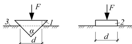
**Figure 4.** Loading of conical and isolated shallow foundations:  $d$ —diameter of conical foundations at the level of the soil base surface; 1—conical foundation; 2—isolated shallow foundation; 3—base soil;  $\alpha$ —cone opening angle.
