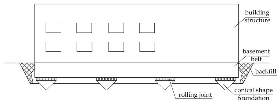
**Figure 3.** Design of a building on conical foundations with deformation joint.
