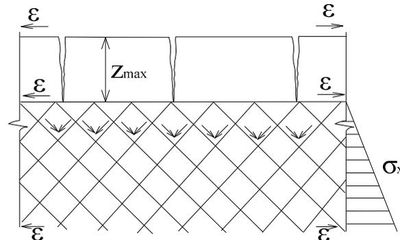
**Figure 2.** Deformations of the sediment layer at the contact with bedrock in the extension zone.
