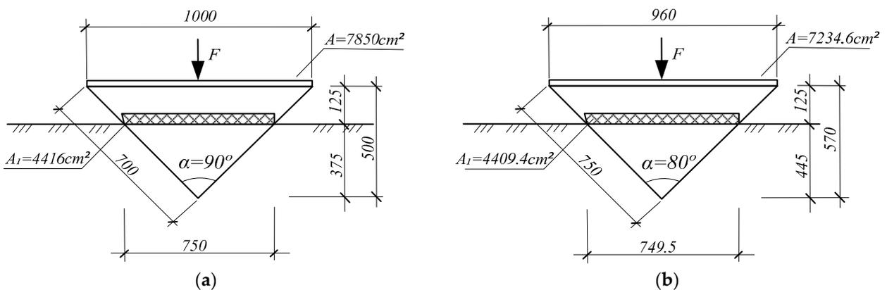
**Figure 8.** Cone shape foundations: (a) with aperture angle  $90^\circ$ ; (b) with aperture angle  $80^\circ$ .
