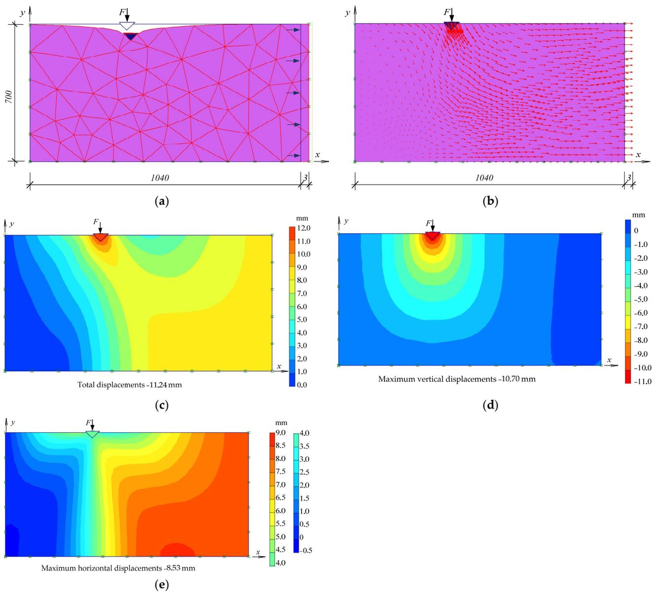
**Figure 11.** Numerical modeling results of a conical foundation with a horizontal soil displacement of 3 mm in the extendable stand: (a) deformed mesh; (b) displacement vectors; (c) total displacement; (d) vertical displacement; (e) horizontal displacement.
