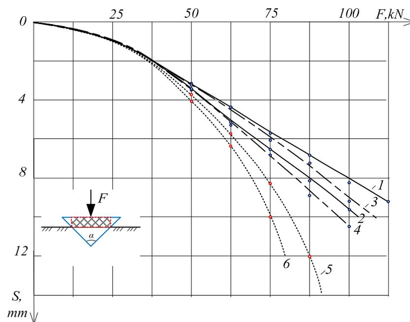
**Figure 14.** Results of full-scale loading tests: 1, 3—curves obtained for horizontal tensile strains  $\epsilon = 0$ , conical foundations with an aperture angle of 90° and 80°; 2, 4—curves obtained for horizontal tensile strains  $\epsilon = 2.6$  mm/m, conical foundations with an aperture angle of 90° and 80°; 5, 6—curves obtained for horizontal tensile strains 0 and 2.6 mm/m for isolated shallow foundations.
