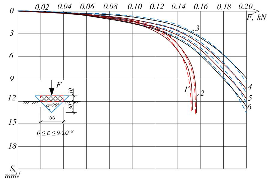
**Figure 15.** Comparison of results of numerical and laboratory methods for conical (with 90° aperture angle) and isolated shallow foundations: 1, 2—curves obtained for isolated shallow foundation with horizontal tensile strains  $\epsilon = 0, 3$  mm/m; 3, 4, 5, 6—curves obtained for conical foundation with horizontal tensile strains  $\epsilon = 0, 3, 6$  and  $9$  mm/m; ----numerical modeling results.
