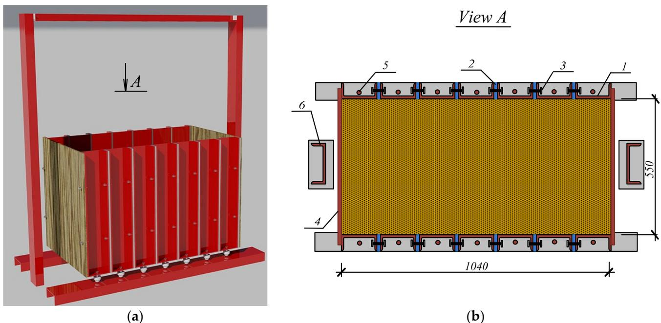
**Figure 5.** Volumetric expandable box: (a) general view; (b) top view, 1—individual channel sections, 2—compressed elastic gaskets, 3—bolted connections, 4—side walls, 5—height-adjustable supports, 6—support frame.
