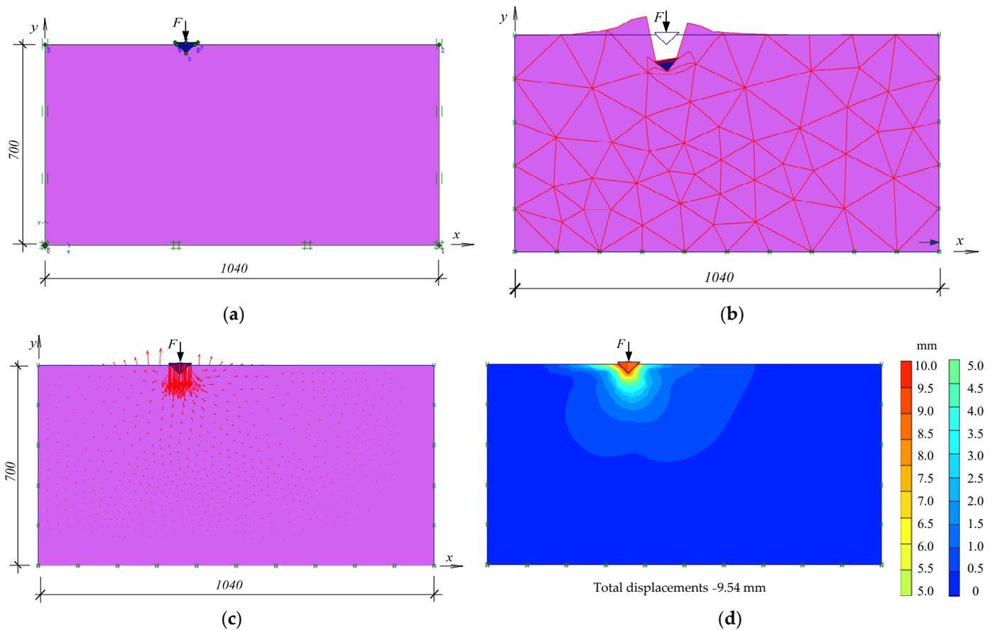
**Figure 10.** Numerical modeling of the conical foundation without horizontal displacement of the soil: (a) setting initial loading parameters; (b) deformed mesh; (c) displacement vectors; (d) total displacement.
