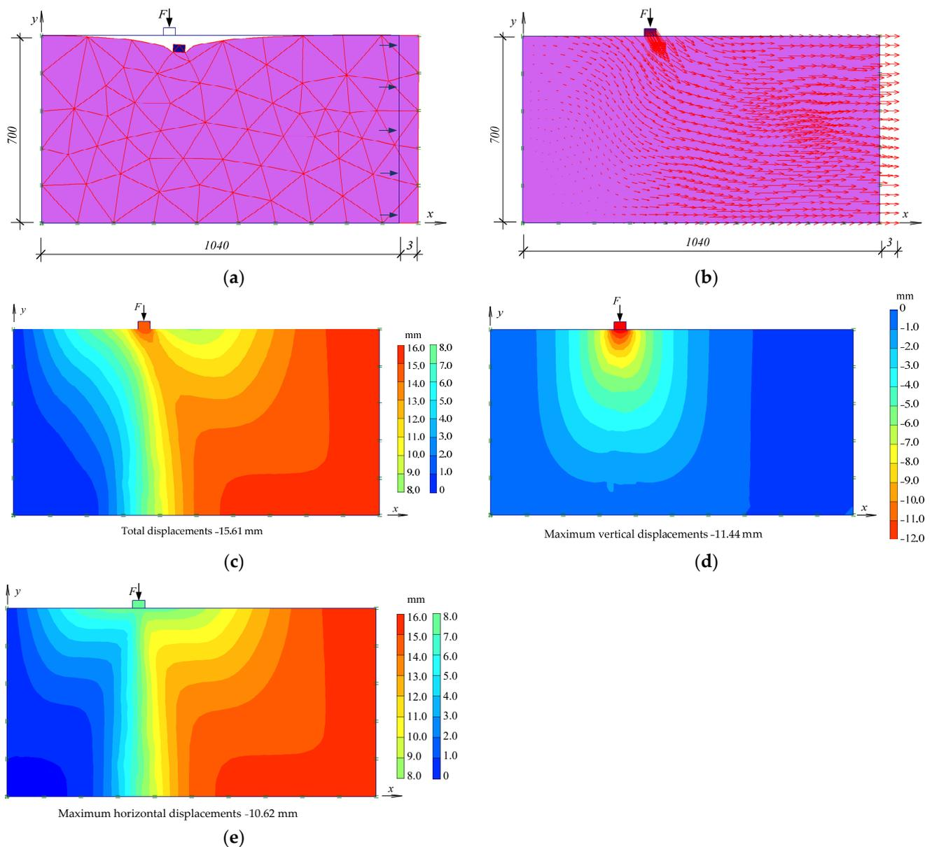
**Figure 12.** Numerical modeling results of an isolated shallow foundation under 0.15 kN load with a horizontal soil displacement of 3 mm in the extendable stand: (a) deformed mesh; (b) displacement vectors; (c) total displacement; (d) vertical displacement; (e) horizontal displacement.
