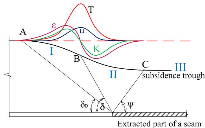
**Figure 1.** The subsidence trough and the distribution of surface deformation:  $\delta_0$ ,  $\delta$  and  $\psi$ —the angles designating the boundaries of the zone of influence of underground mining along the strike of the formation; T—tilt; K—curvature;  $\varepsilon$ —horizontal strain; u—horizontal displacement.
