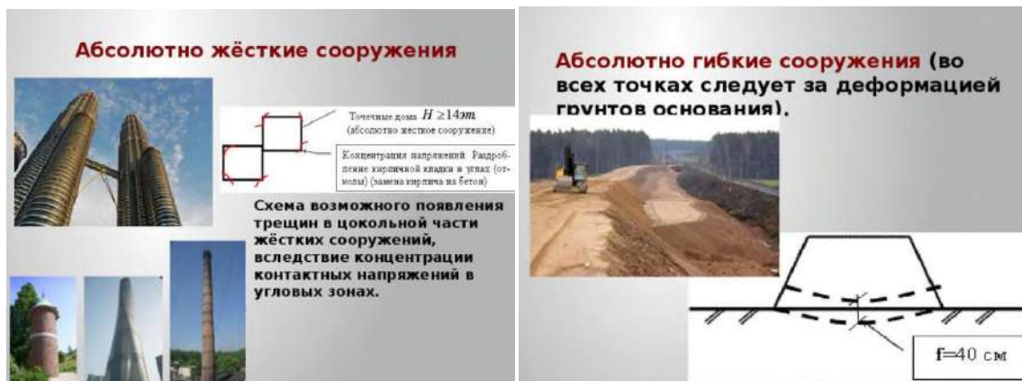
Fig. 3. Absolutely rigid and flexible structures [3]
