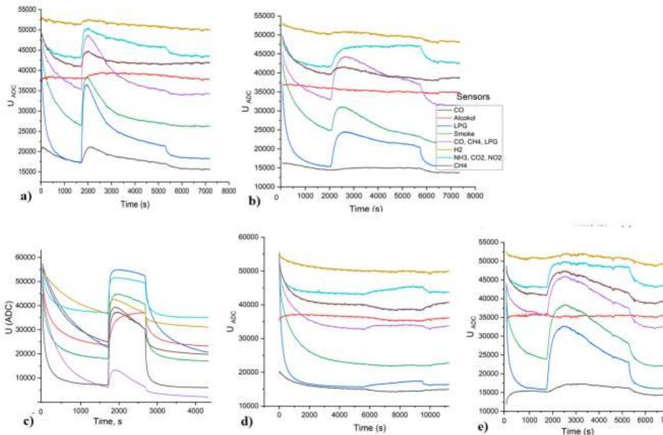
Fig. 2: The time-dependent electrical characteristics of e-nose sensors for PDPs: (a) Gasoline; (b) Diesel fuel; (c) Kerosene; (d) Engine oil; (e) Used engine oil.
