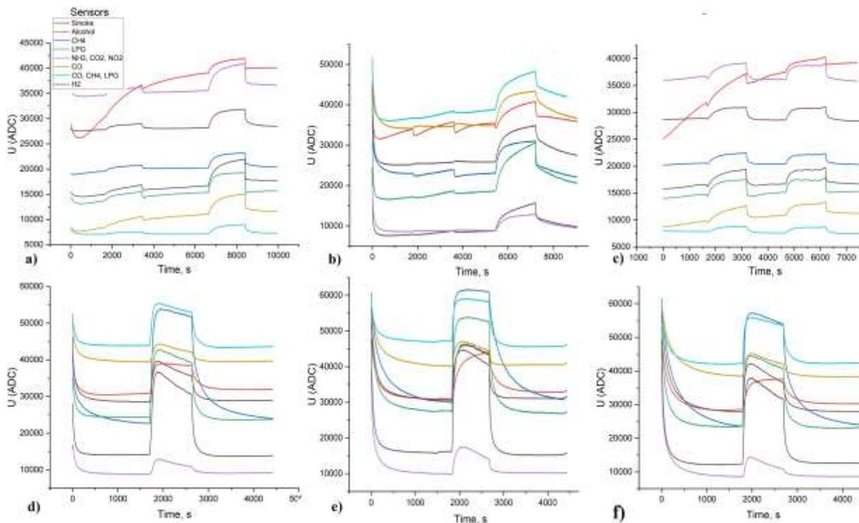
Fig. 3: The time-dependent electrical characteristics of e-nose sensors for the uncontaminated and contaminated soil samples: (a) chernozem (dry and wet), (b) sand (dry and wet), (c) birch grove soil (dry and wet), (d) chernozem sand + kerosene; (e) sand + Kerosene, (f) birch grove soil + kerosene.
