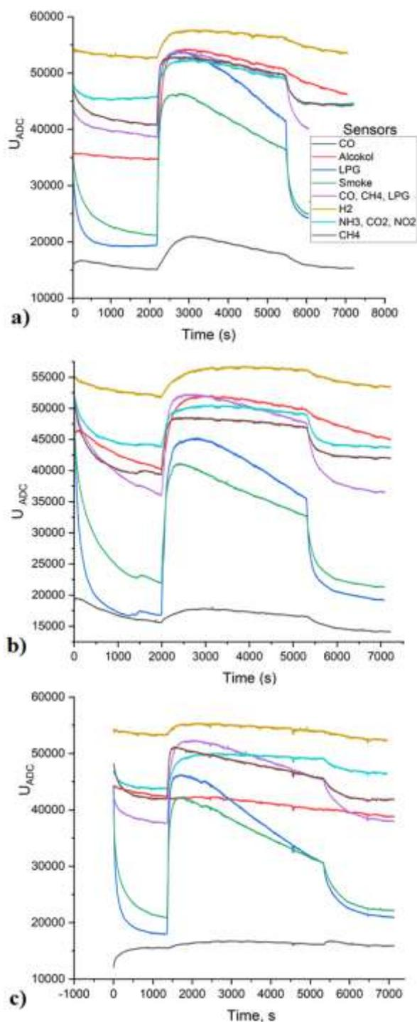
Fig. 1: The time-dependent electrical characteristics of e-nose sensors for crude oil from three Kazakhstan oil fields: (a) Alibekmola, (b) Alibek Yuzhny, (c) Kardasyn North.
