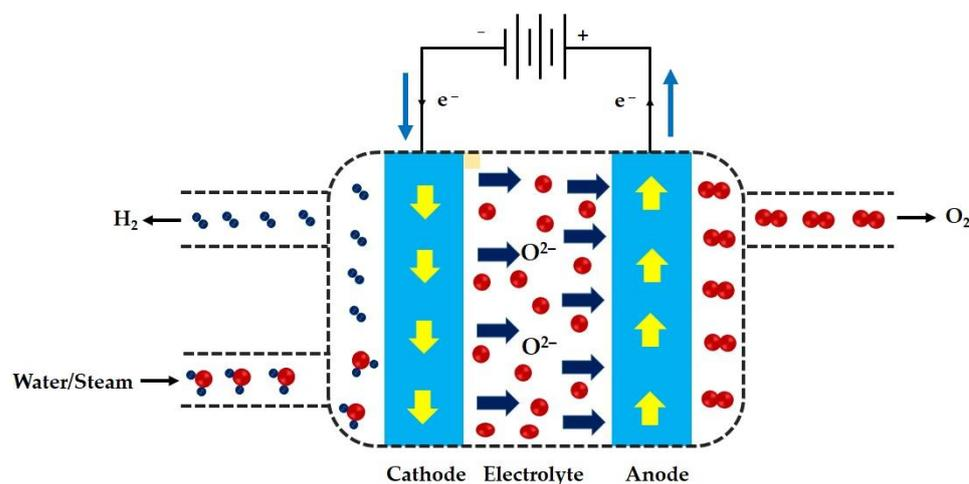
**Figure 1.** A conceptual drawing of a solid oxide water electrolyzer (yellow coloured arrows indicated the flow of electron and blue coloured arrows indicated the flow of oxygen ions) (reproduced from Leonardo Vidas and Rui Castro, 2021) [38].
