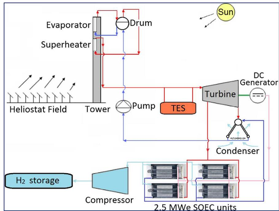
**Figure 4.** General layout of the hybrid SOEC plant with solar towers and hydrogen [78].
