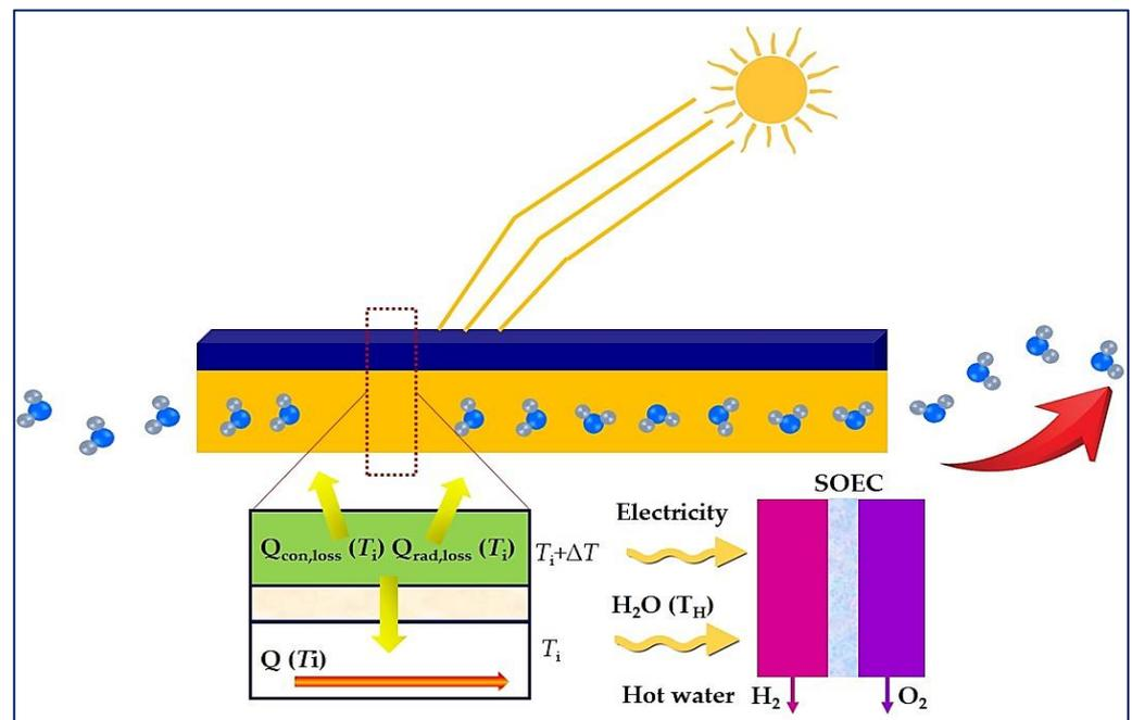
**Figure 5.** Schematic diagram of energy analysis for the heating section (modified from Wang et al., 2020) [6].
