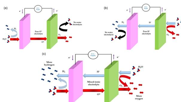
**Figure 3.** Schematic representations of the operating mechanism of (a) oxygen SOEC, (b) proton SOEC, and (c) hybrid SOEC (reproduced from Kim et al., 2017) [50].
