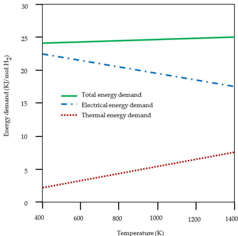
**Figure 2.** Temperature-dependent energy demands for electrolytic H<sub>2</sub> (modified from Ni et al., 2008) [55].
