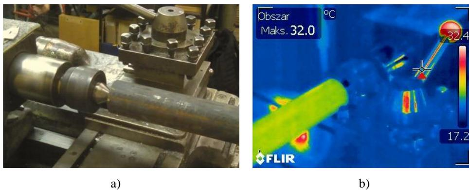
Fig. 2. Thermal imaging laboratory stand: a) the cast iron shaft mounted in the TUD50 lathe, b) thermography image taken with FLIR 335 camera in room conditions temperature
