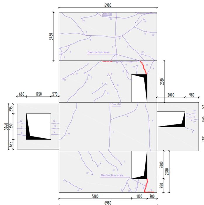
**Figure 24.** Crack scheme in volumetric block M3.
