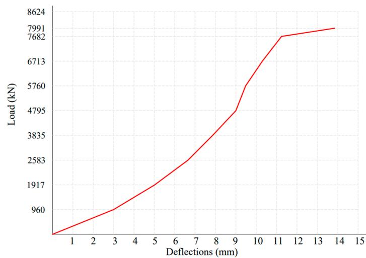
**Figure 39.** Deflections of the floor slab.
