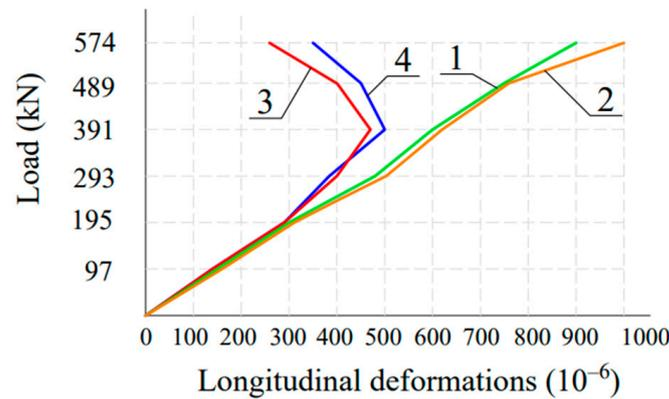
**Figure 26.** Diagram of longitudinal deformations of concrete in the longitudinal wall of a volumetric block: (1, 2) the extreme parts of the longitudinal wall; (3, 4) the middle part of the longitudinal wall.
