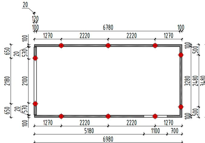
**Figure 7.** Scheme of volumetric block M1 with jacks along the perimeter of the walls.
