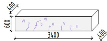
Figure 19. Cracks in the transverse beam of the stylobate.
