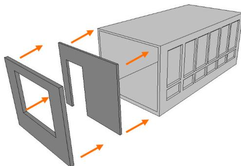
**Figure 1.** Scheme of the block “lying glass”.
