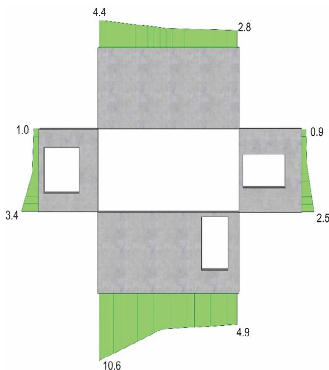
**Figure 40.** Horizontal displacements from the wall plane.
