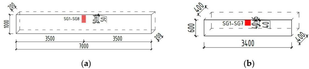
Figure 4. Arrangement of strain gauge: (a) on the longitudinal beams of the stylobate; (b) on the transverse beam of the stylobate.
