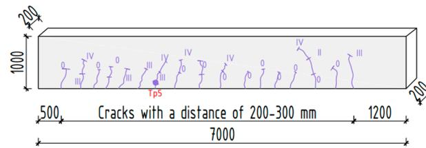
Figure 30. Diagram of the location of cracks in the longitudinal beam of the stylobate.
