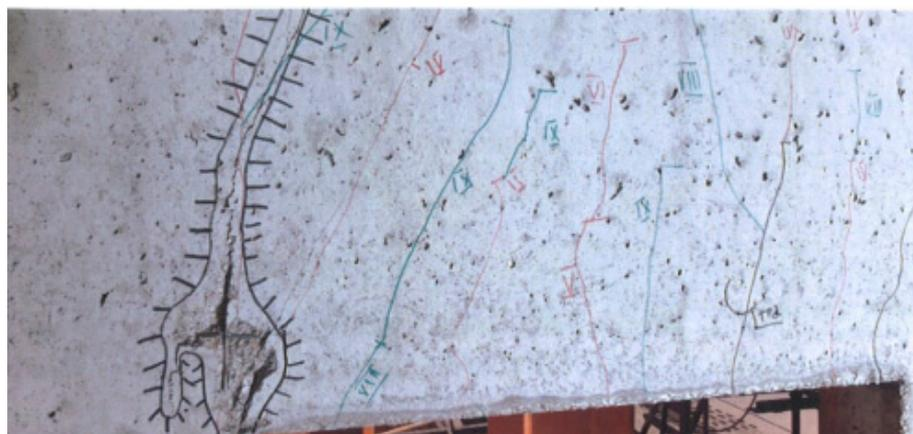
**Figure 25.** Failure of the longitudinal wall lintel with a change in the crack banks.
