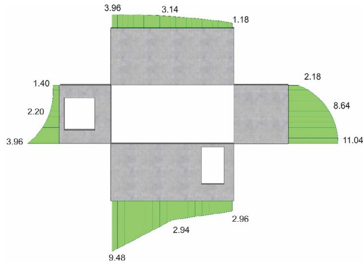
**Figure 9.** Horizontal deformations (deplanation) of the walls of the volumetric block under a vertical load of  $N = 4795$  kN, mm.
