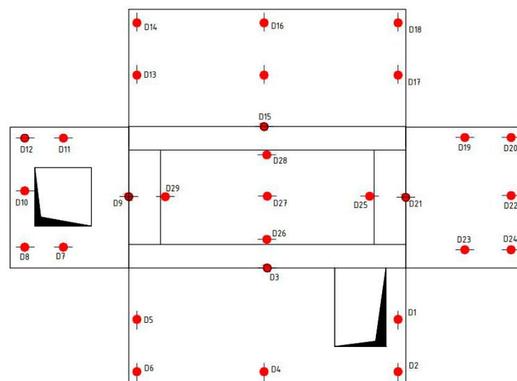
Figure 5. Scheme of horizontal and vertical arrangement of deflection indicator.
