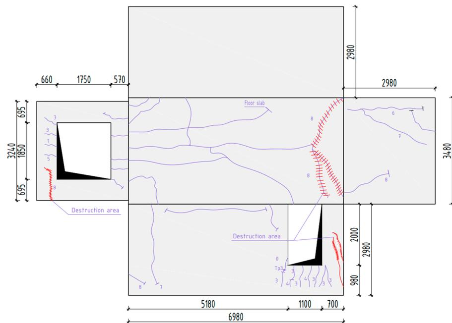
**Figure 14.** Crack scheme.
