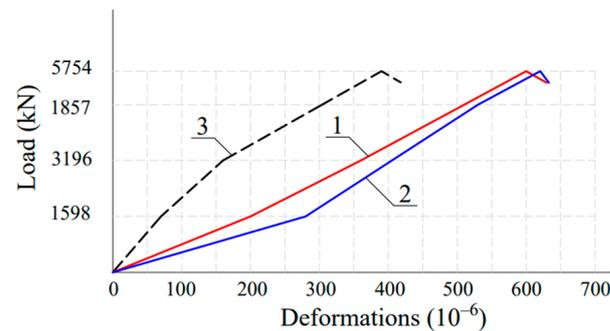
**Figure 17.** Diagram of compressive deformations in walls: (1, 2) the extreme parts of the wall; (3) the middle part of the wall.
