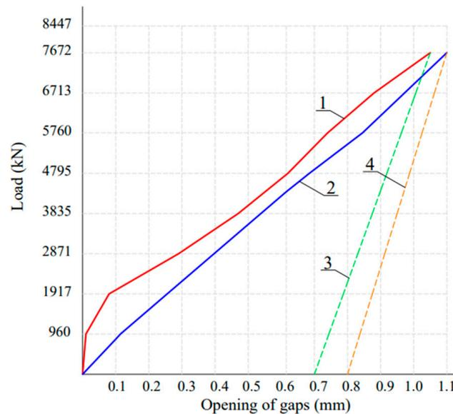
**Figure 34.** Width of the opening of the gaps under longitudinal walls: (1, 2) between the stylobate and the longitudinal walls; (3, 4) residual cracks after removal of loading.
