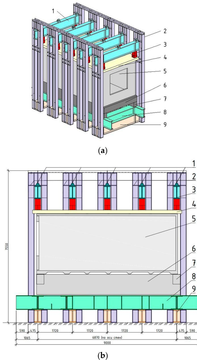
**Figure 2.** Scheme of an experimental facility with stylobate beams and a volumetric block (a) façade and (b) section: (1) PM-3 frame; (2) PM-2 frame; (3) jacks; (4) distribution slab; (5) test block; (6) secondary beam; (7) main beam; (8) frame PM-1; (9) base frame.
