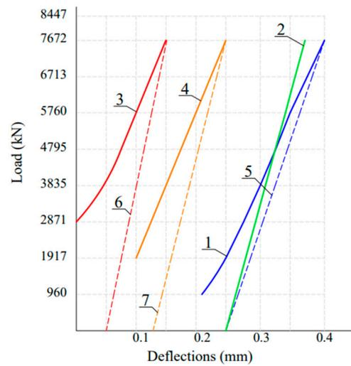
**Figure 37.** Cracks in stylobate beams: (1, 2) longitudinal beams; (3, 4) transverse beams; (5, 6, 7) residual cracks after removal of loading.
