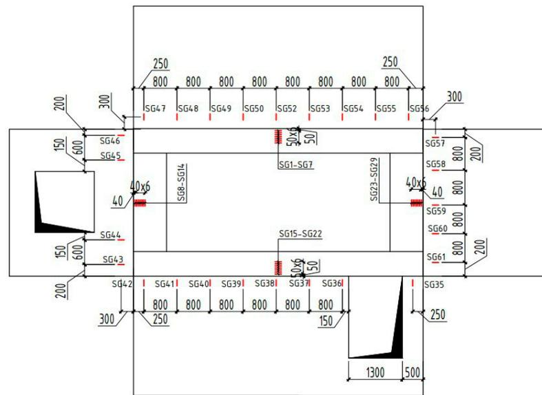
Figure 3. Scheme of the load strain gauge on the walls of the volumetric block.
