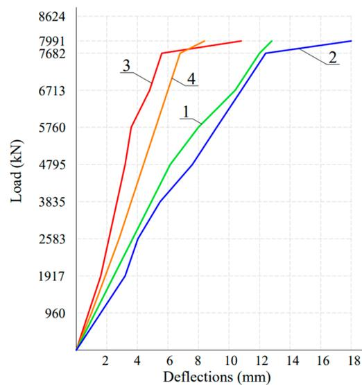
**Figure 38.** Walls deflections: (1, 2) longitudinal walls; (3) end wall; (4) wall panel.
