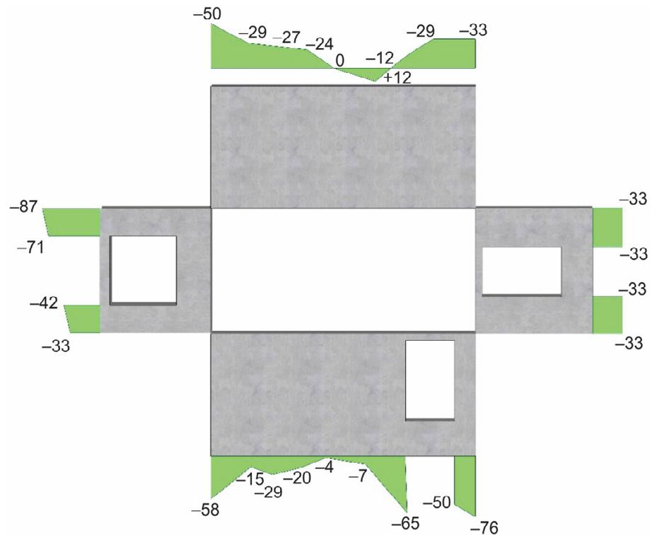
**Figure 28.** Concrete strains in the walls of the volumetric block.
