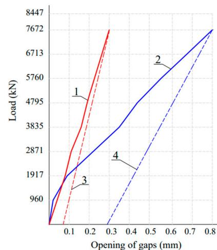
**Figure 35.** Opening the width of the gaps under the end wall and the wall panel: (1) end wall; (2) wall panel; (3, 4) residual cracks after removal of loading.
