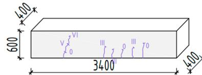
Figure 31. Diagram of the location of cracks in the transverse beam of the stylobate.
