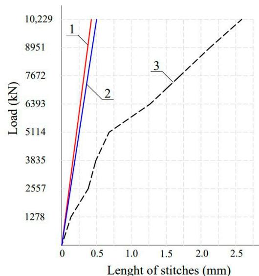
**Figure 12.** The opening of the gap between the longitudinal walls and beams of the stylobate and the deflections of the floor slab: (1, 2) between the stylobate and the longitudinal walls; (3) deflections in the floor slab of the volumetric block.
