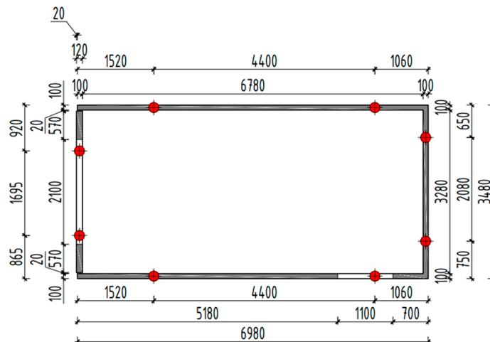
**Figure 10.** Arrangement of hydraulic jacks modeling with wind effect.
