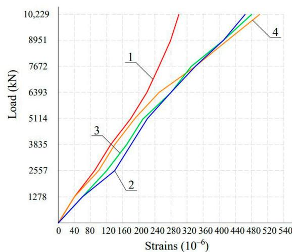
**Figure 11.** Concrete strains in longitudinal walls under a vertical load of  $N = 5347$  kN: (1, 2) longitudinal wall; (3, 4) the extreme part of the longitudinal wall.
