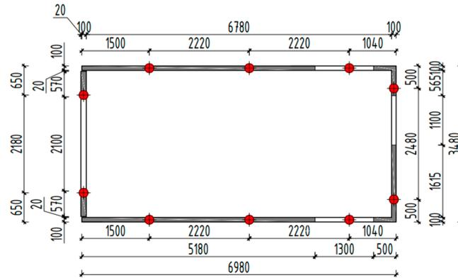
**Figure 23.** Scheme of volumetric block M3 with jacks placement.
