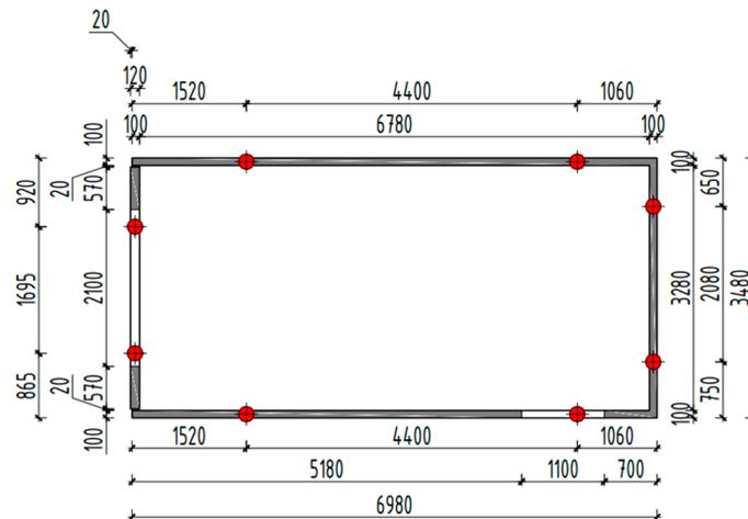
**Figure 15.** Scheme of replacement jacks.
