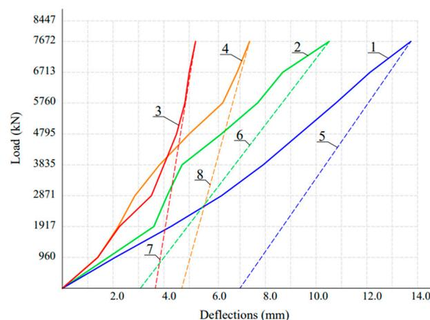
**Figure 36.** Deflections of the walls of the volumetric block: (1, 2) longitudinal walls; (3) end wall; (4) wall panel; (5, 6, 7, 8) residual cracks after removal of loading.
