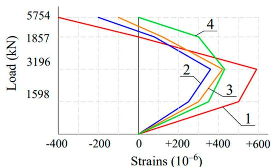
**Figure 21.** Diagrams of concrete strains in the upper part of the longitudinal beam of the stylobate: (1, 2, 3, 4) the deformation of the strain gauges along the height of the beam during the maximum destructive load.
