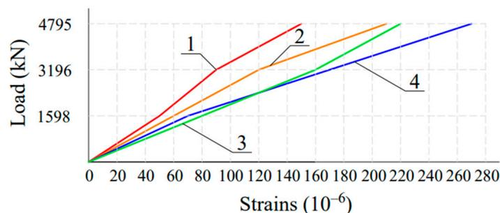
**Figure 8.** Concrete strain diagram for the longitudinal walls of a volumetric block: (1, 2) the middle part of the wall; (3, 4) the extreme part of the wall.
