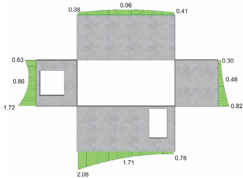
**Figure 13.** Horizontal displacements (deplanation) of the walls, mm.
