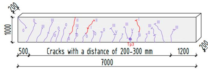
Figure 18. Cracks in the longitudinal beam of the stylobate.
