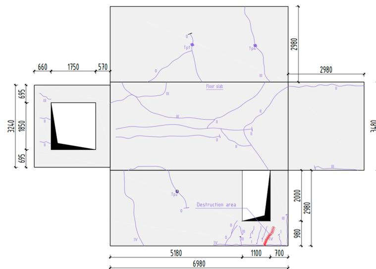
Figure 20. Scheme of cracks in the volumetric block.
