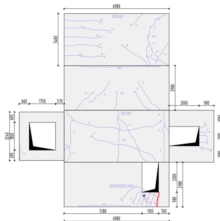
**Figure 29.** Scheme of cracks in the volumetric block M4.
