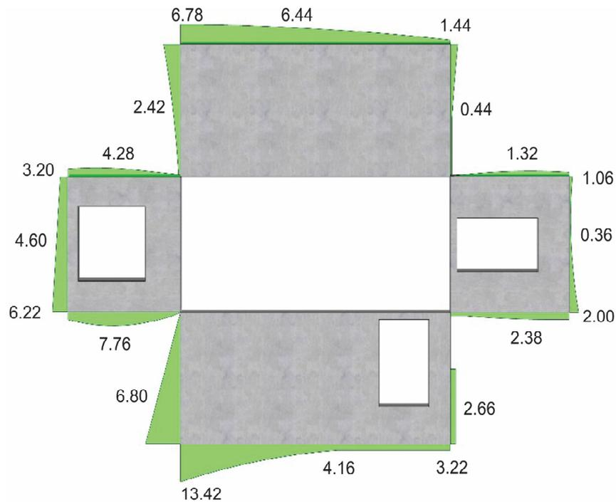
**Figure 27.** Horizontal displacements (deplanation) of the walls, mm.
