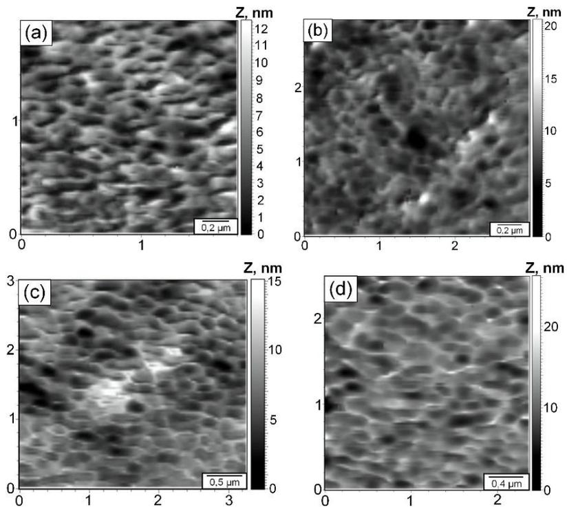
**Figure 2.** AFM images of the samples: (a) PETF-100; (b) PETF-100/Nafion; (c) PETF-100/Nafion<sub>dil.</sub>; (d) PETF-100/(Nafion + npSiO<sub>2</sub>).
