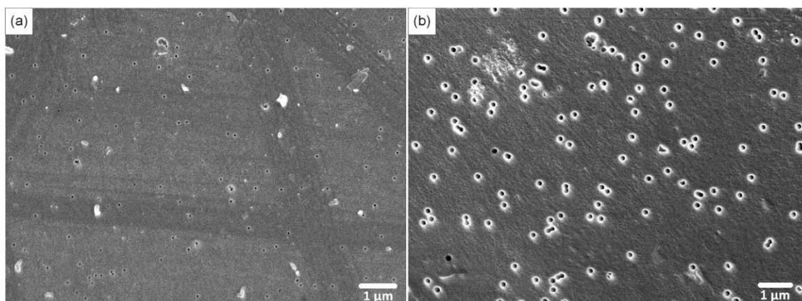
**Figure 4.** SEM-images of structure of surfaces PETF-membranes with diameter of pores of (a) 100 nm and (b) 200 nm, modified by layer of Nafion with SiO<sub>2</sub> nanoparticles.
