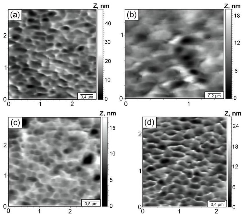
**Figure 3.** AFM images of the samples: (a) PETF-200; (b) PETF-200/Nafion; (c) PETF-200/Nafion<sub>dil.</sub>; (d) PETF-200/(Nafion + npSiO<sub>2</sub>).
