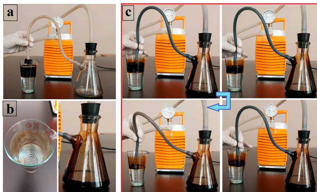
Figure 10. Continuous separation of oil and water using a superhydrophobic PU/MgFe 2 O 4 /RGO/SO magnetic sponge (40 wt% loading) and a diaphragm vacuum pump, (a) before separation; (b) after separation; (c) during separation.
