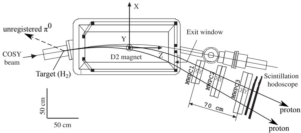
Figure 1. Forward detector of the ANKE spectrometer.
