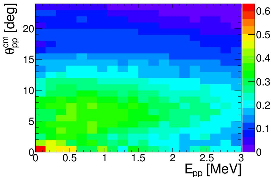
Figure 7. Effective acceptance of detector  $A$  with respect to the excitation energy of the proton pair  $E_{pp}$  and its angle in the c.m.s.  $\theta_{pp}^{cm}$  for the reaction  $pp \rightarrow \{pp\}_s \pi^0$ .
