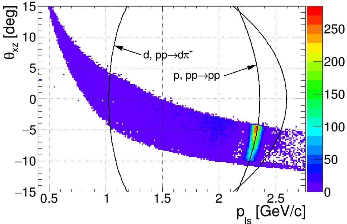
Figure 4. Momentum-angular acceptance of the forward detector ( $T_p = 1.6$  GeV).
