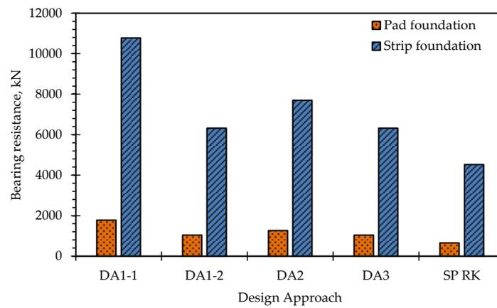
**Figure 5.** Comparison of the values of bearing capacity for pad and strip foundations adhering to Kazakhstani and European approaches.
