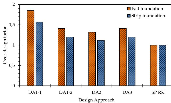
**Figure 7.** Comparison of the values of over-design factor for pad and strip foundations adhering to Kazakhstani and European approaches.
