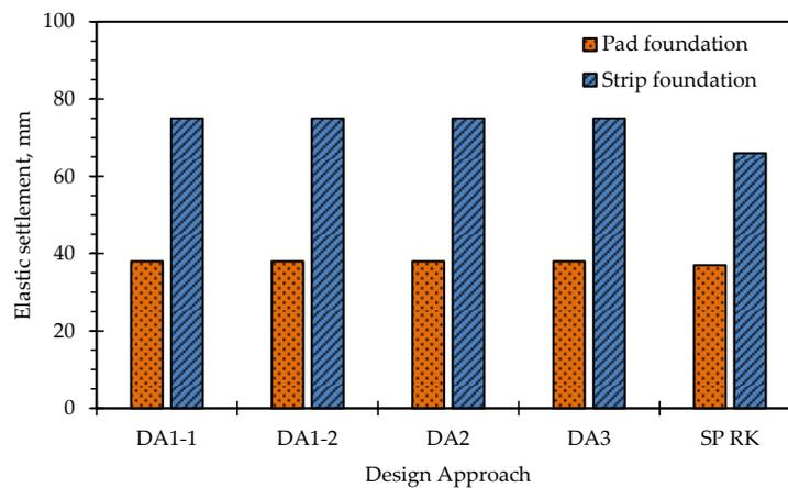
**Figure 6.** Comparison of the values of elastic settlement for pad and strip foundations adhering to Kazakhstani and European approaches.
