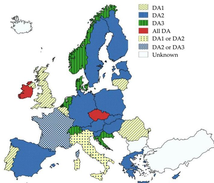
**Figure 2.** Design Approaches in the European member states for the design of shallow foundations.
