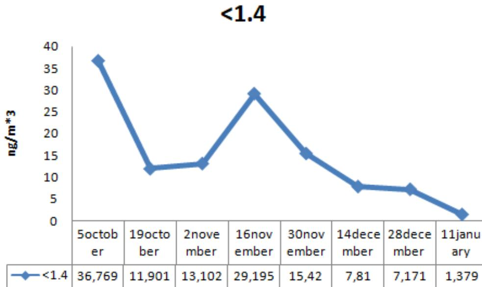
Figure 10. The level of radioactivity of manganese for a filter of size <1.4  $\mu\text{m}$ .
