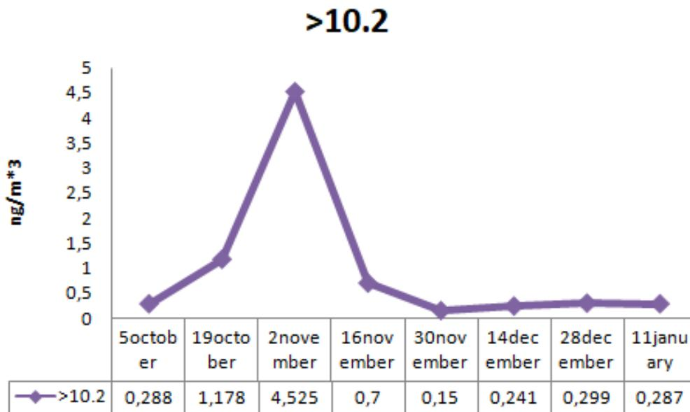
Figure 6. The level of radioactivity of manganese for a filter of size >10.2  $\mu\text{m}$ .
