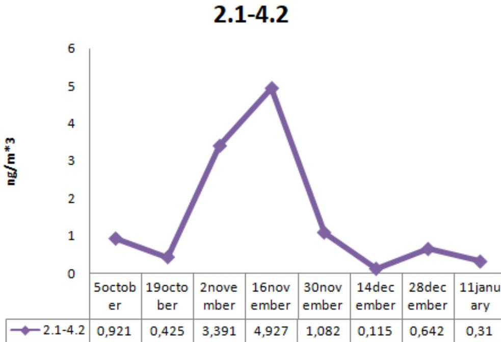
Figure 8. The level of radioactivity of manganese for a filter of size 2.1-4.2  $\mu\text{m}$ .
