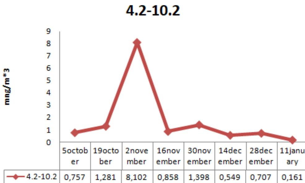
Figure 7. The level of radioactivity of manganese for a filter of size 4.2-10.2  $\mu\text{m}$ .
