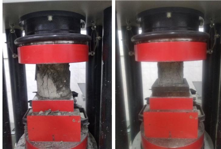
**Figure 2.** Compression test of cylindrical and cubic samples on the 1st, 3rd, 7th, 14th and 28th days.
