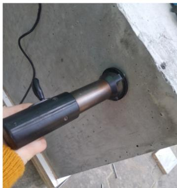
**Figure 4.** Determination of the strength of concrete in boxes obtained by the IPS-MG 4.01 sclerometer.
