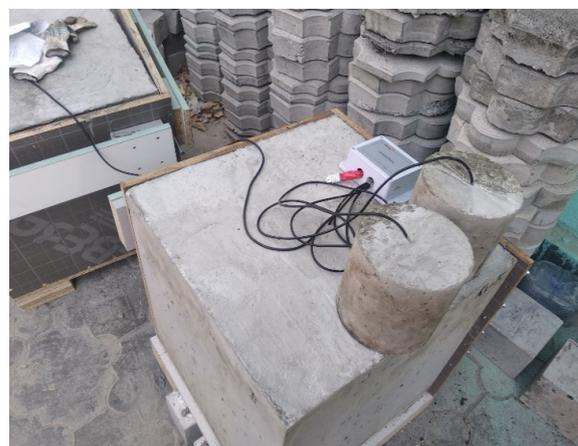
**Figure 1.** Testing set for estimating the concrete strength.
