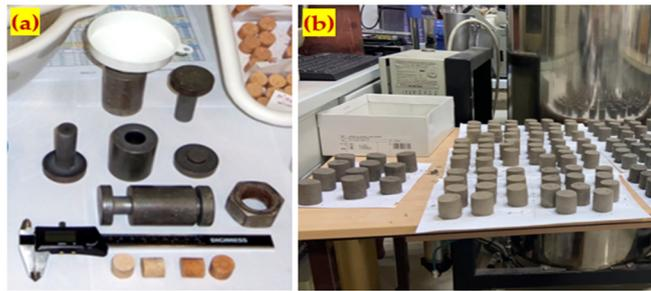
**Figure 2.** Details of specimen preparation: (a) tools used for compaction; (b) appearance of compacted specimens.
